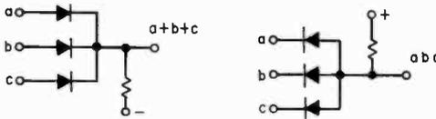
Logic is performed by diodes. The output is not inverted. Amplifiers are required to maintain the correct logic levels through several gates in series.
