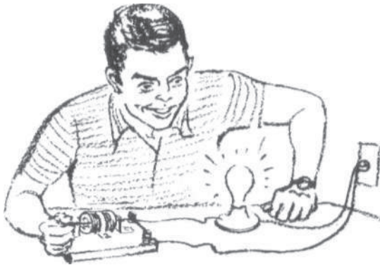
Fig. 607. A lamp dimmer is constructed by connecting a 15-watt 117-volt electric light in series with a solenoid. Withdraw the plunger in the solenoid, the lamp glows; insert it, the lamp gets dimmer.
