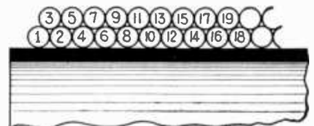
Method of bank winding wire on a coil form.
