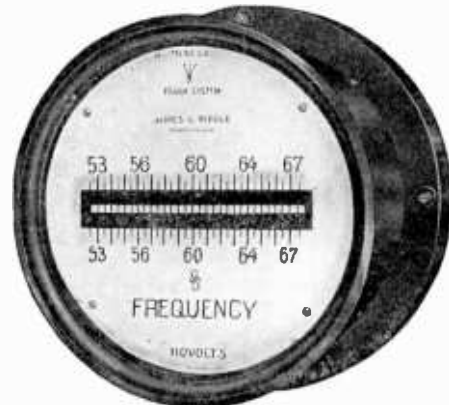
Illustration by Courtesy of Jas. G. Biddle. A vibrating reed type of frequency meter.
