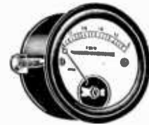
Panel-type of voltmeter.
