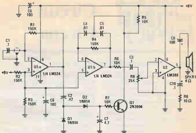
Fig. 2. This circuit is similar to the circuit in Fig. 1, except that the signal detected by the capacitor sensor is used to trigger the circuit.
