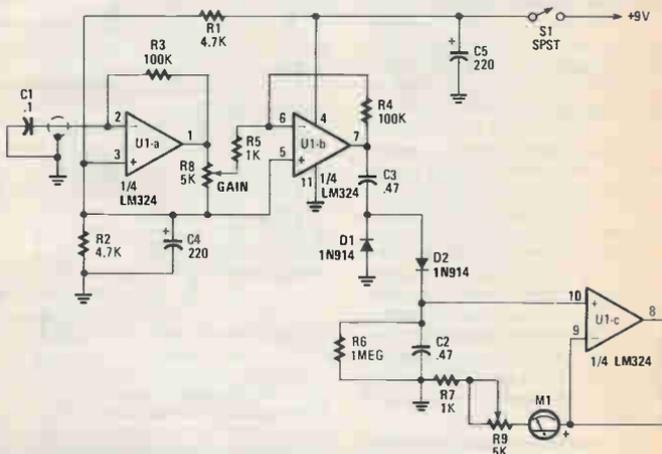
Fig. 3. Here is a circuit that should be of interest to car buffs and others involved with tracking down the source of strange knocking noises in electro-mechanical devices.
