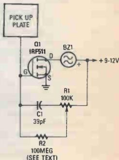
Fig. 3. The sensitivity of this Proximity Switch can be varied by adjusting R1. Note that R2 is specified as a 100-megohm unit, if that value cannot be located tie five 22-megohm resistors in series and use that combination for R2.
