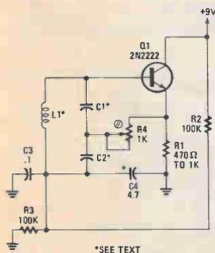
Fig. 2. This oscillator is designed to operate at a much higher frequency than the previous circuit, and its upper frequency limit is governed primarily by the transistor.
