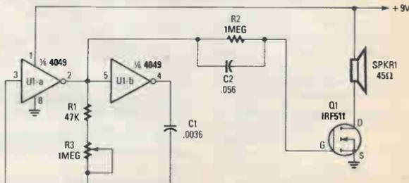
Fig. 5. This simple VFO circuit can be used for audible-tone testing, driving someone nuts, or it can be transformed into a simple electronic musical instrument—an electronic organ, for example.
