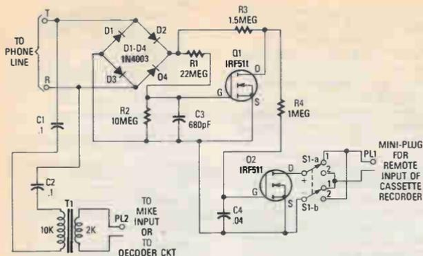
Fig. 6. The Cassette Interface does not require its own power supply, but instead rectifies a portion of the incoming audio signal to provide power for the circuit.
