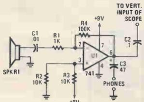
Fig. 4. In the receiver section of the distance-measuring system, a single 741 op-amp (U1) is wired as an inverting amplifier and is used to boost the level of the incoming signal by a factor of about 100.
