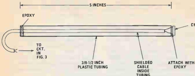
Fig. 4. Shown here are construction details for the probe unit used with the knock-detector circuit.
