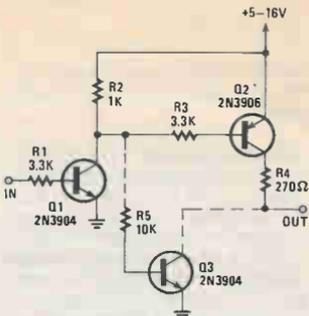
Fig. 10. The non-integrated buffer, like its integrated counterparts, can be used to increase the output drive current.
