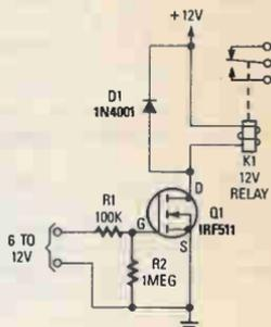
Fig. 2. With zero gate-bias applied, Q1 acts like an open switch, but when a DC voltage greater than 5 volts is applied to the input of the circuit, Q1 turns on, completing the relay circuit, and thereby activating the relay.
