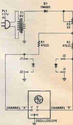
Fig. 3. The Oscilloscope-Based Matching Circuit allows you to look at the forward conduction curve of both diodes simultaneously on an oscilloscope.
