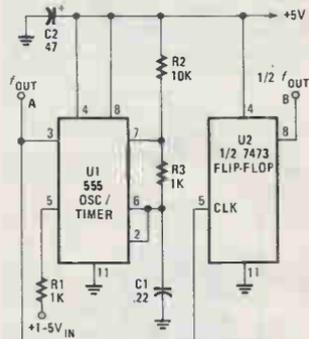
Fig. 3. In this circuit, a 555 oscillator timer is used as a simple VCO. The signal produced by the VCO is fed to U2 (half of a 7473 dual TTL flip-flop), which provides a square-wave output that varies at half the input frequency.
