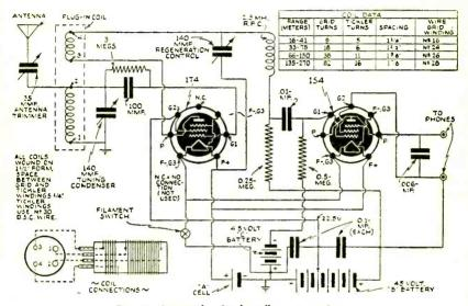
Fig. 1-Circuit for 2-tube all-wave receiver.
