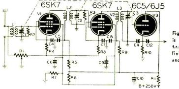
Fig. 5—Tuner is a 3-tube t.r.f. with infinite-impedance detector.
