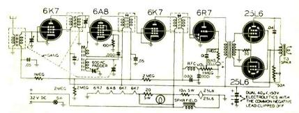
Fig. 1—Schematic diagram of the 32-volt receiver. I. f. is 455 kc.
