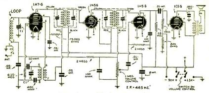
Fig. 1—Set wired for battery operation.
