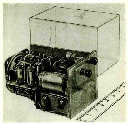
The "Miniport"—a 5-tube battery portable.
