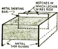
Fig. 7—Sliding block used to short Lecher wires.
