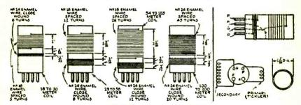
Fig. I-Coil winding data for Twinplex.
