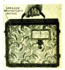
Panel of 4-tube broadcast band portable.
