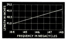
Fig. 8—This chart shows the frequency for a given distance between nodes on the Lecher wire system.
