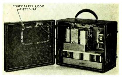
Rear view, with lid open, showing batteries.
