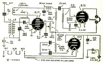
Wiring diagram of the "Midget 3-Tuber".
