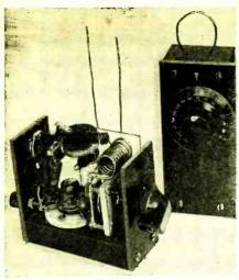
Front view of 955 receiver and wavemeter.
