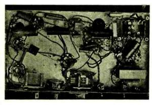
Bottom view of short-wave superhet receiver. Wiring and parts are not crowded. The low cost of the parts is rather due to the use of double-purpose tubes, and to the design of the circuits around tubes which require a minimum of circuit components.
