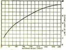
Fig. 1—Antenna height for given radio range.
