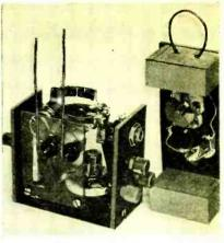
Above—Rear view of receiver and wavemeter. The receiver employs a 955 acorn tube connected in a superregenerative circuit. This set is ideal for mobile use with batteries.
