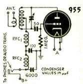
Fig. 2—The receiver is a superregenerator.
