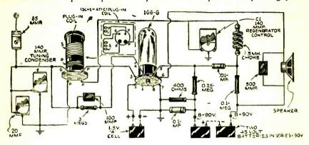
Fig. 2-Diagram of one-tube receiver.
