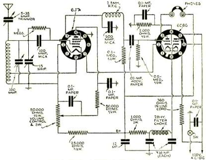
Fig. 1—Circuit of 2-tube beginner's receiver.
