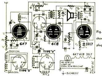
Fig. 1 — Schematic shows switching and plug-in combined.
