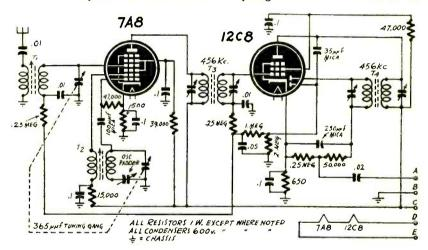
Schematic. The connections between the two sections of the diagram are keyed A-A, B-B, etc. Consider these solid connections when tracing circuits from one section to the other.
