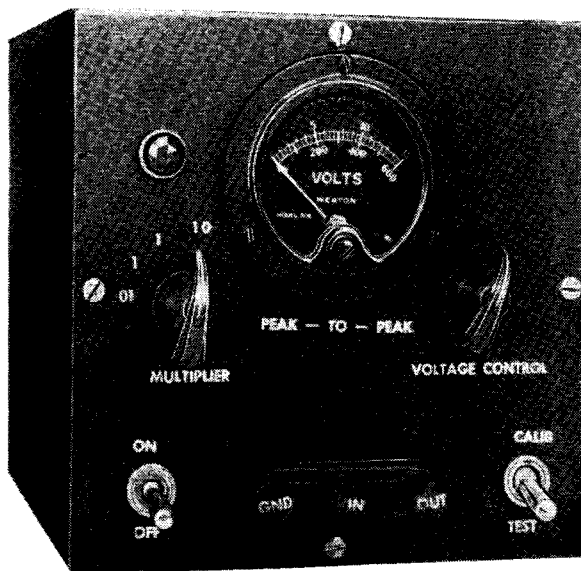
Fig. 702. Front panel photo of the peak-to-peak voltage calibrator. The meter can have a full-scale deflection of 1.5 ma or less.
