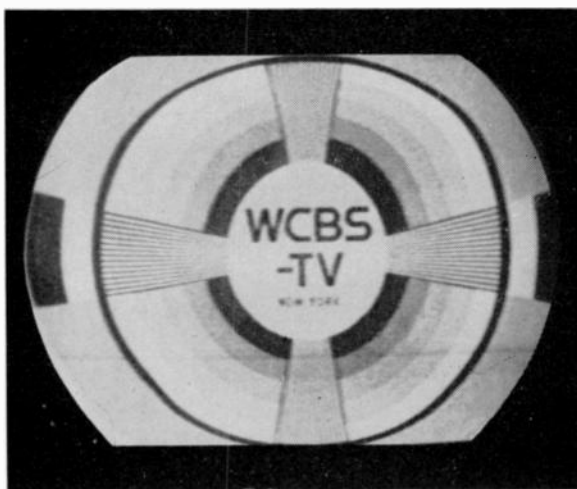
Fig. 1401. Photo above shows blurred pattern due to line reflections.
