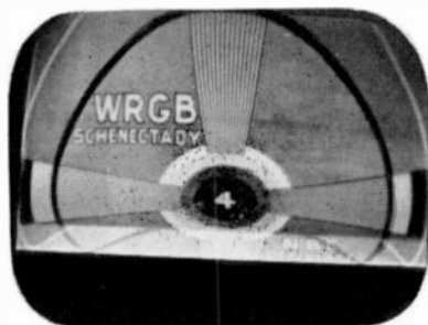
Fig. 1203. Foldover at bottom of picture.
