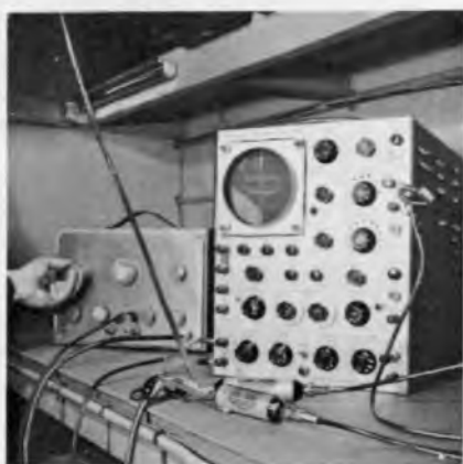
Fig. 412. Photo of test setup utilizing dual crystal probes instead of a balanced probe.
