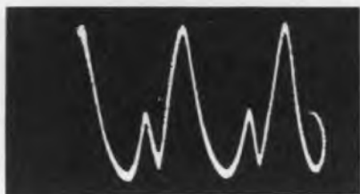
Fig. 116. Waveform with two components. A v.t.v.m. can indicate the voltage of the larger component, but does not reveal the presence of the smaller one.
