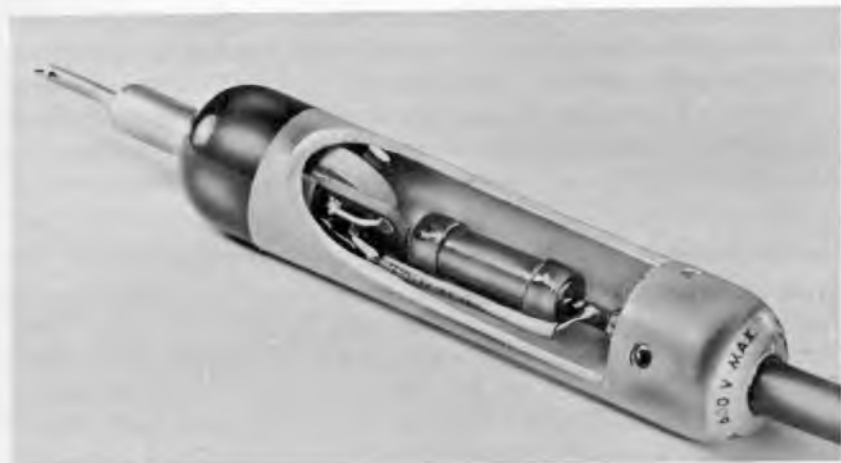
Fig. 507. Cut-away view of the interior of a low-capacitance probe showing placement of parts.
