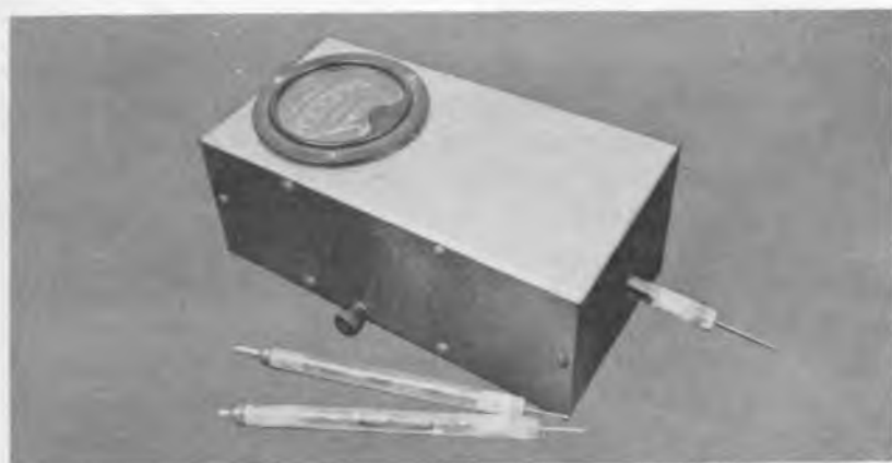
Fig. 813. Photo of the trim-looking unit and the associated plug-in multiplier probes. The positioning of the meter is not critical and may be turned to suit your convenience. An inexpensive 0-1 ma meter is used.
