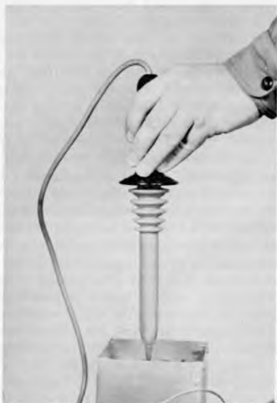
Fig. 617. Correct technique for using a high-voltage probe.
