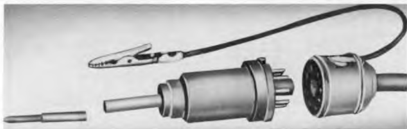
Fig. 1017. Photo of the vacuum-tube probe. The probe is very sensitive and can be used in very low r.f. signal voltage stages.
