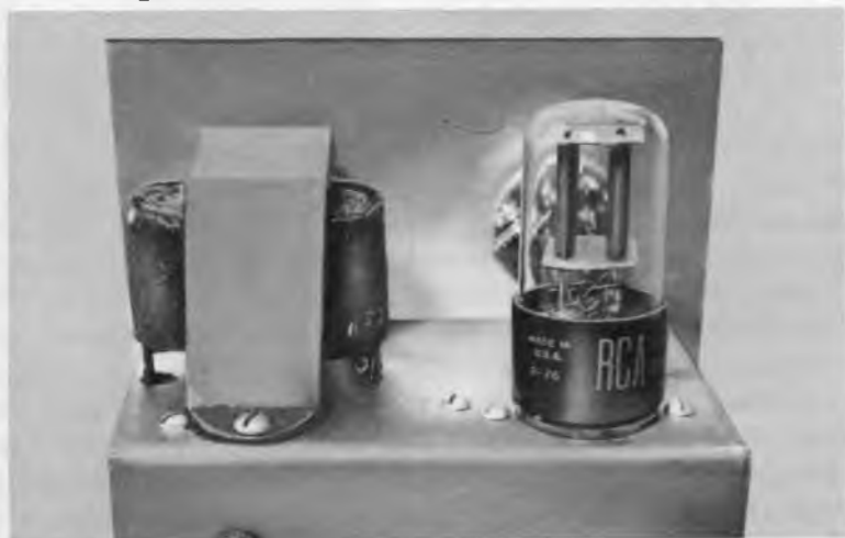
Fig. 113. Top view of the preamplifier. Either an open- or shielded-type power transformer can be used. Amplifier uses but a single tube.
