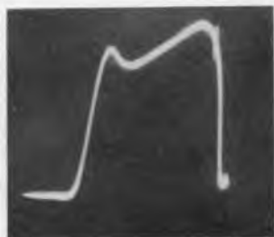
Fig. 205. A typical scope pattern observed when tracing a sweep signal through the input stages of a TV i.f. amplifier.
