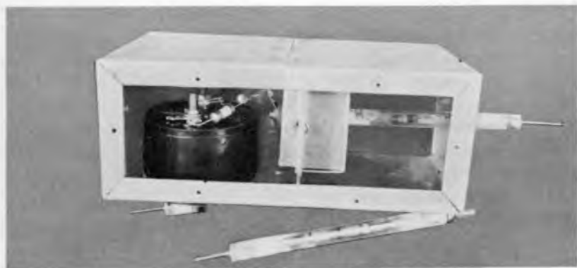
Fig. 814. View of the inner construction showing placement of the components. The metal box consists of two shielded compartments. Both sides of the metal housing are held in place by self-tapping screws. The entire probe is readily accessible for any repairs or changes you might wish to make.
