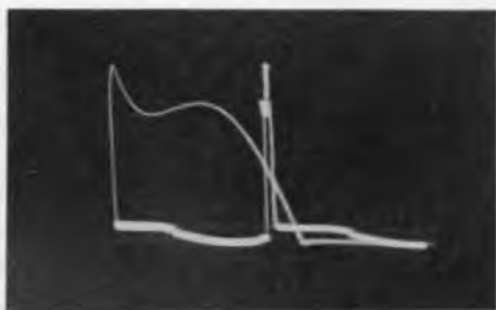
Fig. 614. Normal 6-kv flyback pulse at plate of horizontal-output amplifier. The capacitance-divider probe attenuates the pulse by a factor of 100 to 1 to avoid damaging the scope input circuit.
