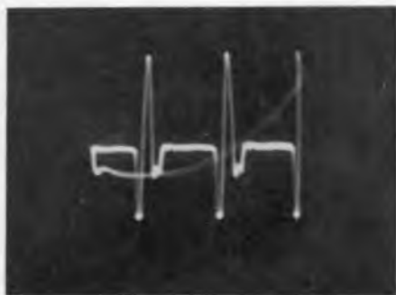
Fig. 610. Negative pulse in sweep-output waveform indicates excessive leakage reactance in flyback transformer, may also generate Barkhausen oscillations.
