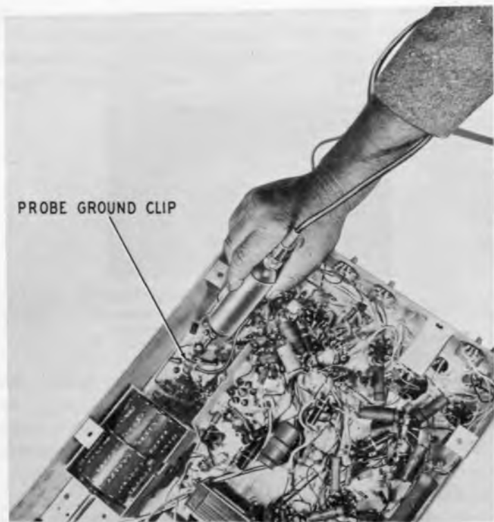
Fig. 105. Signal tracing in a TV i.f. amplifier with a crystal demodulator probe. Note probe ground clipped to chassis as close as possible to signal take-off.
