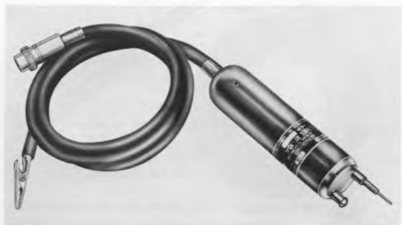
Fig. 1004. Probe comes equipped with two grounding points. The stud on the probe head should always be used when making tests in high-frequency circuits.
