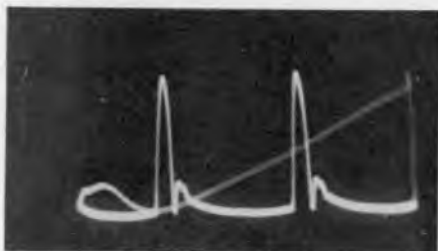
Fig. 609. Normal sweep waveform at the plate of horizontal-output tube, seen with the aid of a 100-to-1 capacitance-divider probe. Diagonal line is scope retrace. Peaks are about 6,000 volts high.
