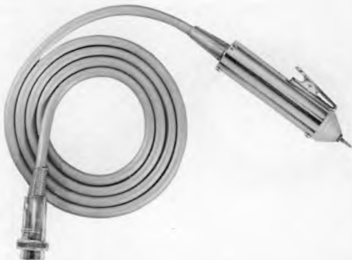
Fig. 1005. This r.f. probe uses a subminiature tube. The clip, fastened to the head of the probe, permits simultaneous grounding and clip-on action.
