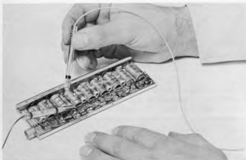
Fig. 811. This picture shows the miniature probes at work. These probes have the advantage of compactness but lack of shielding limits usefulness.
