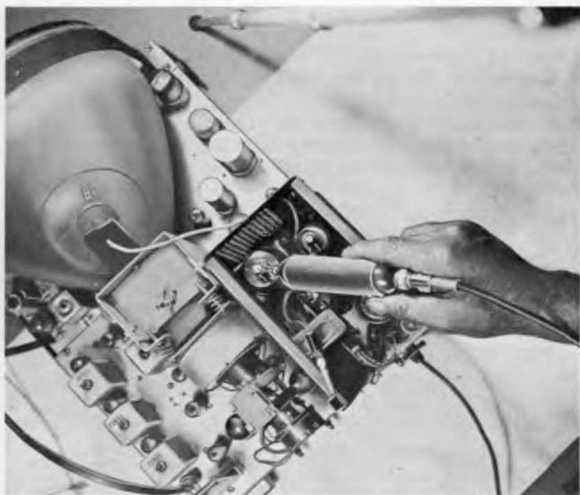
Fig. 602. Photo shows capacitance-divider probe being used to check high voltage waveforms.
