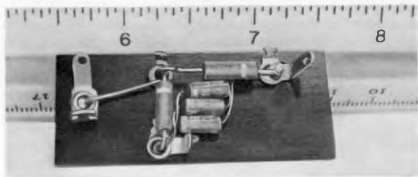
Fig. 902. Internal layout of the Chromatic Probe. The three crystals form a non-linear network. The output of the probe is the difference between the two signals that are applied to the probe input.
