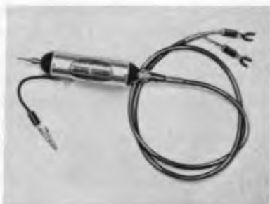
Fig. 107. Probe and output leads must be shielded to prevent pickup of undesired signals.
