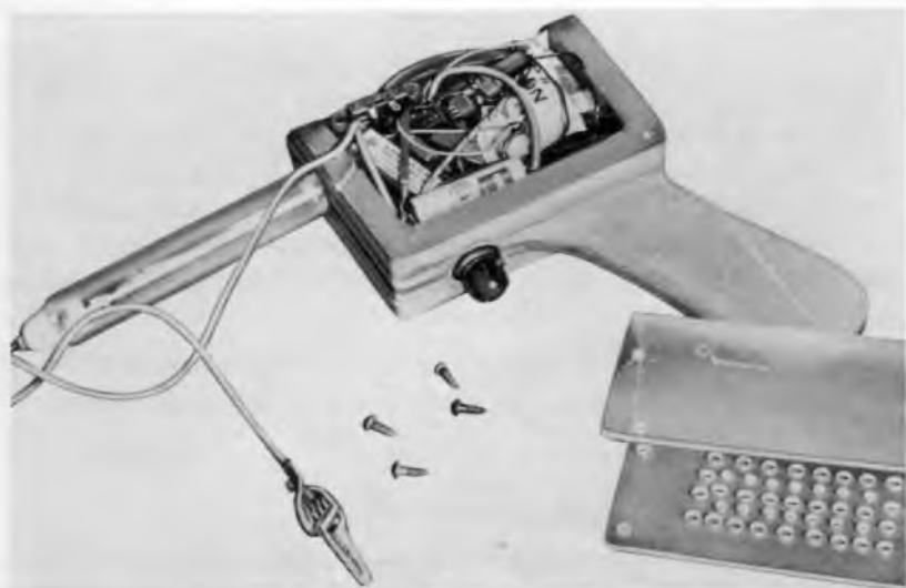
Fig. 826. Assembly of the transistor probe. The plastic cover, held on by four wood screws, has a large number of drilled holes which act as a speaker grille.
