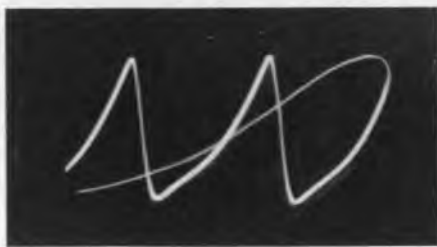
Fig. 516. Distorted current waveform in horizontal yoke indicates trouble in sweep circuit.
