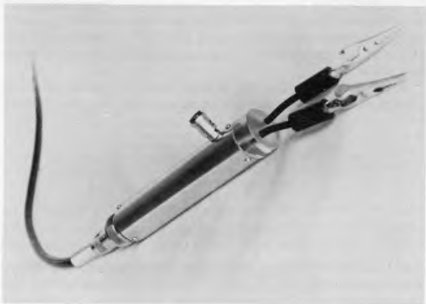
Fig. 414. Photo of balanced probe. The ground connector is fastened to the probe housing.
