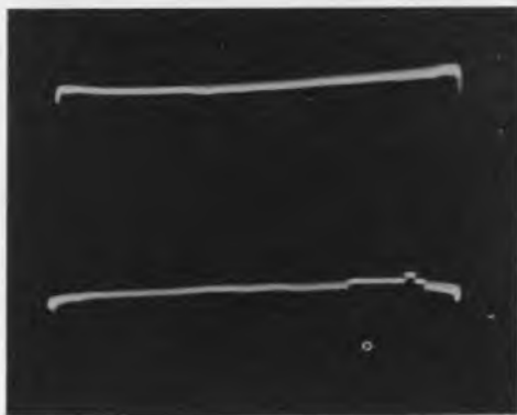
Fig. 405. Curvature in the zero-volt reference line, sometimes noted during impedance checks of lead-ins and antennas, or front ends of TV receivers, is caused by 60-cycle pickup in the balanced crystal probe. Grounds should all be returned to a common point, and thence to a cold-water pipe. Ground all instrument cases.
