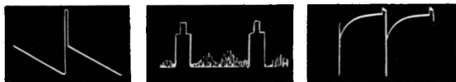
Fig. 115. A properly calibrated scope will enable you to measure the amplitudes of these TV waveforms.
