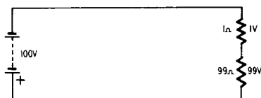
Fig. 606. Simple resistive network illustrates probe action.
