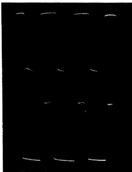
Fig. 515. Output waveform of one-shot multivibrator, 10 volts p-p.
