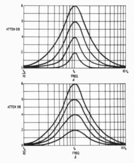
Fig. 627-a, -b. Families of curves for equalizer circuits.
