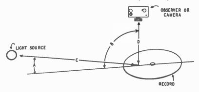
Fig. 916. Setup for visual groove inspection.
