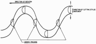
Fig. 915. Illustration of pinch effect.
