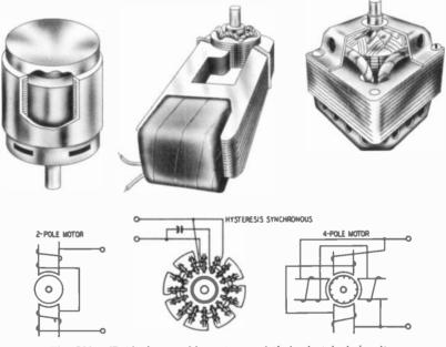
Fig. 901. Typical turntable motors and their electrical circuits.
