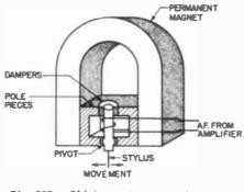
Fig. 909. Chief components of a magnetic cutter.
