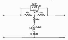
Fig. 626. Here we have the final circuit of the equalizer whose design was calculated and described for you in the text.
