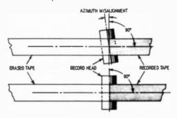
Fig. 930. Angular displacement of the record head will produce distortion.
