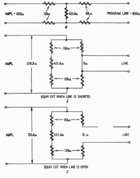
Fig. 605-a, -b, -c. Attenuators can be used as isolation networks.
