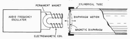
Fig. 702. Movement of the diaphragm, caused by the varying current through the coil, produces sound.
