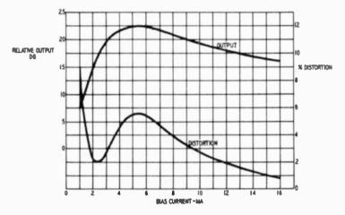
Fig. 928. Effect of bias current on output and distortion.
