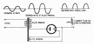
Fig. 405. The line voltage is stepped up by the transformer and is rectified by the diode. The output consists of pulses.
