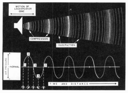
Fig. 102. The motion of the cone of a loudspeaker produces changes in the pressure of the air surrounding the cone.
