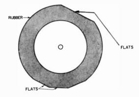
Fig. 504. Flat spots in phono idler wheel produce sound distortion.
