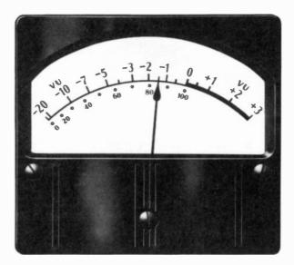
Fig. 206. Volume-unit meter. The upper scale indicates VU and the lower scale shows percentage of modulation.
