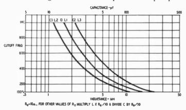
Fig. 723. Design curves based on the networks of Fig. 722.
