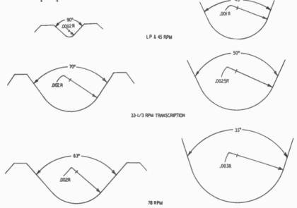
Fig. 907. Record groove dimensions (left) and stylus dimensions (right). These drawings are not to scale, and are exaggerated for the sake of clarity.
