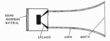
Fig. 710. Typical horn-type loudspeaker.
