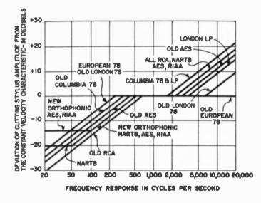
Fig. 912. Typical recording characteristics.
