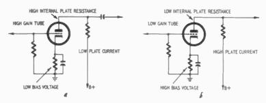
Fig. 308-a,-h). The circuit at the left is a voltage amplifier; that at the right is a power amplifier. The circuits are drawn the same way, but component values and type of operation differ.
