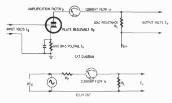
Fig. 325. The vacuum-tube amplifier can be simplified to an equivalent circuit.
