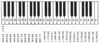
of harmonics. The fundamental sine wave combines with the harmonics to produce complex waveforms. It is the presence of these harmonics which gives the piano its particular tone. Frequencies other than harmonics are produced when a key is struck, but the harmonics are the most important. This means that an gudio system must be able to pass a wide range of frequencies.
