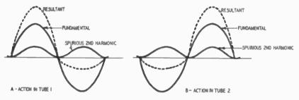
Fig. 319-a-b. Waveforms in the output of a push-pull circuit.
