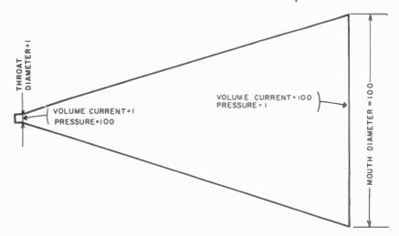
Fig. 713. Relationship of throat and mouth pressures in a horn.
