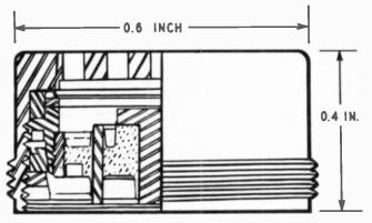
Fig. 814. Extremely small size is unique feature of this condenser microphone.
