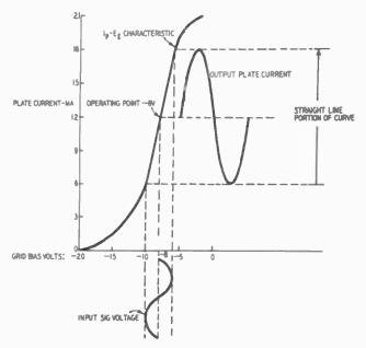
Fig. 301. The class-A amplifier produces an undistorted output waveform but is characterized by very low efficiency.
