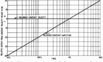
Fig. 911. This curve also shows a 6 db slope per octave. Compare this with Fig. 910.
