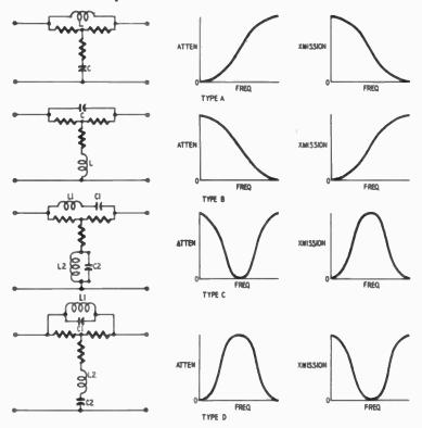
Fig. 623. Equalizer networks and their attenuation and transmission characteristics.
