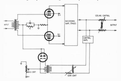
Fig. 323. In this circuit we have a volume compressor added to a typical push-pull unit.
