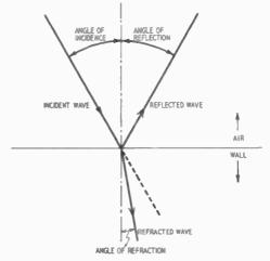
Fig. 101. Sound, striking a wall, is reflected by it. Some of the sound is absorbed by the wall and a portion of the sound is transmitted by it.
