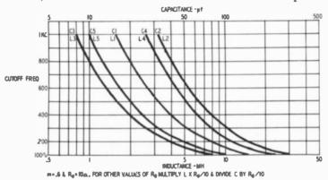
Fig. 721. Family of characteristic curves of crossover networks.
