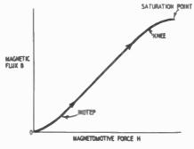
Fig. 921. Normal magnetization curve.
