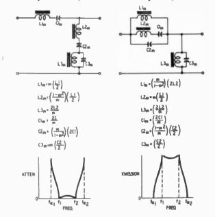
Fig. 619. M-derived half section used as a bandpass filter.
