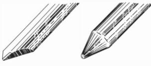
RECORDING STYLUS PLAYBACK STYLUS Fig. 905. Difference in construction between recording and playback styli.
