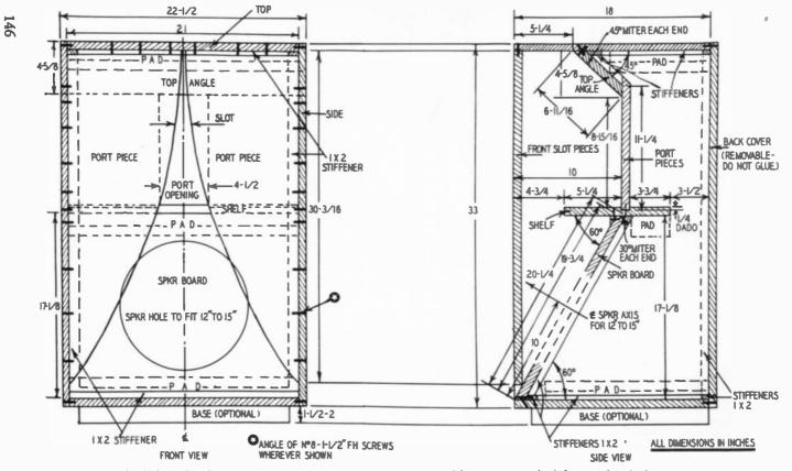
Fig. 709. This loudspeaker enclosure works on the musical-instrument principle of a closed pipe.
