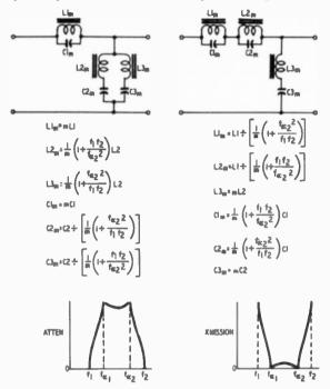
Fig. 620. M-derived half section used as a band elimination filter.
