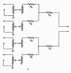
Fig. 610-c. Series-parallel mixer circuit.
