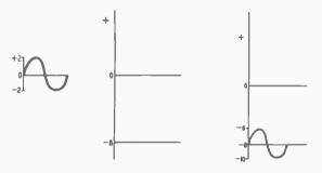
Fig. 302. The signal voltage (left) added to the d.c. bias (center) gives us an a.c. wave with a d.c. component, (right).
