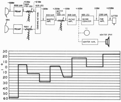
Fig. 205. Block diagram of an audio-amplifier system. The graph indicates the loss or gain of the various units in the system.
