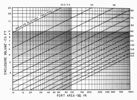
Fig. 705. This chart gives the relationship between the volume, resonant frequency and port area of a bass-reflex enclosure.
