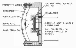
Fig. 803. Crystal microphone in cross-section.
