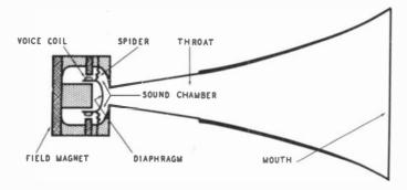
Fig. 712. The horn acts as an acoustic transformer.
