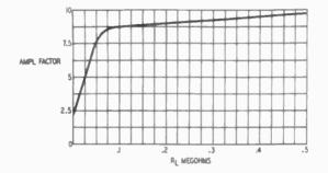
Fig. 315. The gain of an audio circuit increases as the resistance or impedance of the load is raised.
