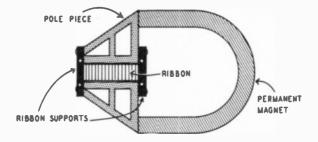
Fig. 806. Velocity or pressure-gradient microphone.
