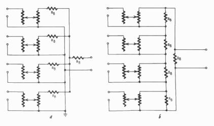
Fig. 610-a. b. Circuit arrangements for mixer type attenuators.
