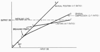
Fig. 324. Characteristics of an amplifier using volume compression.
