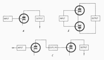
Fig. 307-a,-b,-c. The circuits shown in a and b provide only a single stage of amplification. In c we have a cascade arrangement of two stages of amplification.
