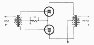
Fig. 318. Fundamental diagram of a push-pull circuit. Center-tapped transformers are used.
