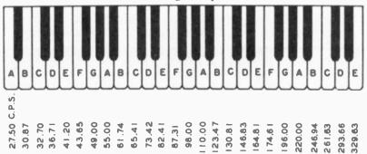
Fig. 103. This illustration shows a standard 88-note piano keyboard. The figures placed below each key indicate the frequency in cycles per second of each corresponding note. Middle A on the piano has been fairly well standardized at 440 cycles per second (c.p.s.). The piano, in common with all other musical instruments, produces complex tones. These tones consist of sine waves plus a number
