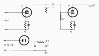
Fig. 310. Elementary audio-amplifier system. Triodes are used here for the sake of simplicity.
