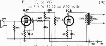
Fig. 328. The final design of the amplifier.
