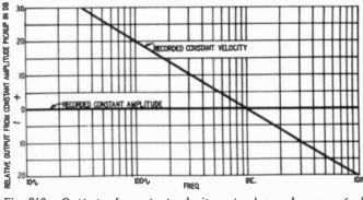
Fig. 910. Output of constant-velocity reproducer decreases 6 db per octave when used with a record made under conditions of constant amplitude.
