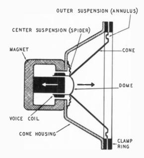
Fig. 703. Cross-sectional view of a dynamic speaker. Most speakers are of the permanent-magnet type.
