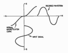
Fig., 925. Distortion produced in recorded waveform.
