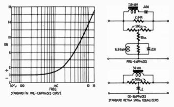
Fig. 621. Typical pre-emphasis and de-emphasis networks. The pre-emphasis curve is used for FM broadcasting.
