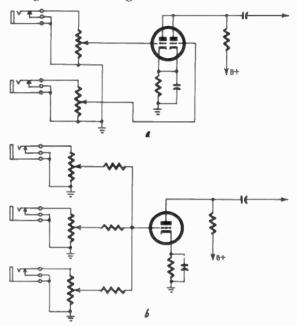
Fig. 609-a, -b. Attenuators can be used for proper mixing of signals.
