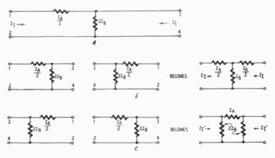
Fig. 611-a, -b, -c. The L-pad can be used to build a T- or pi attenuator.
