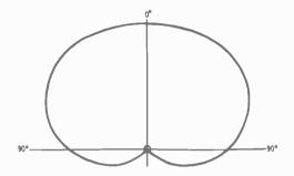
Fig. 808. Graph of a cardioid characteristic.
