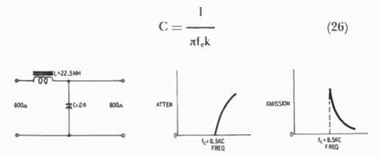
Fig. 612. Single constant-k I. section showing attenuation and transmission characteristics.
