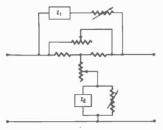
Fig. 628. Basic arrangement of a constant-B equalizer circuit.
