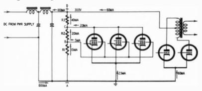
Fig. 411. The power supply furnishes plate and screen voltages for the tubes. The tubes may be considered as a load in parallel with the output of the power supply.
