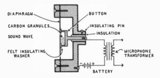
Fig. 801. Cross-sectional view of carbon microphone.
