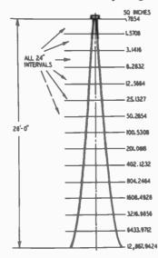
Fig. 716. Design of a horn.
