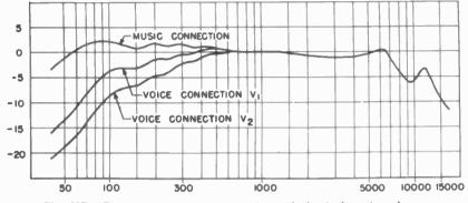
Fig. 807. Frequency response curves of a typical velocity microphone. ance unaffected by temperature, humidity or variations in atmospheric pressure.
