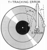
Fig. 904. Error produced by angular motion of pickup arm.
