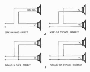
Fig. 718-a, -b. Proper phasing of speakers is important.
