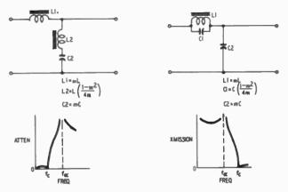
Fig. 617. M-derived half section. M is usually taken as 0.6.
