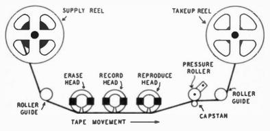
Fig. 923. Major components of a tape recording system.
