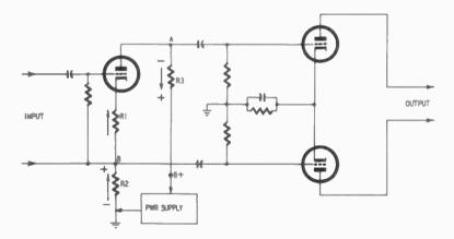
Fig. 320. A single tube can be used to supply out-of-phase signals for driving tubes in push-pull.
