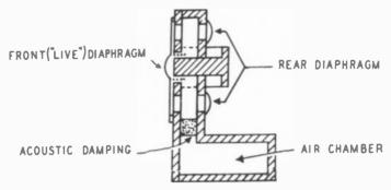
Fig. 812. In this microphone the acoustic air chamber is below the microphone.
