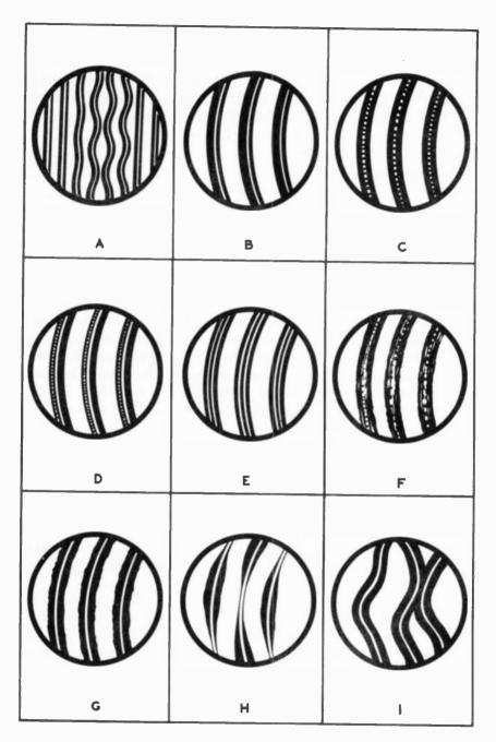
Fig. 920. Typical faults revealed by microscopic examination of the grooves of a record.
