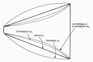
Fig. 714. This illustration shows shapes of typical horns.
