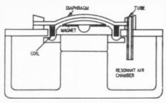
Fig. 804. Dynamic or moving-coil microphone.
