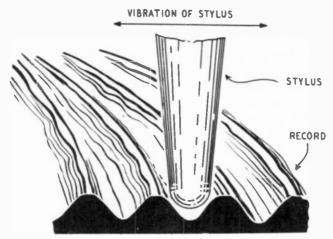
Fig. 908. Stylus is supported by walls of the groove.
