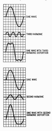
Fig. 502. Effect of second and third harmonic distortion on a sine wave.
