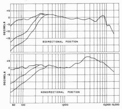
Fig. 810. Several of the frequency response characteristics of the microphone illustrated in Fig. 809.
