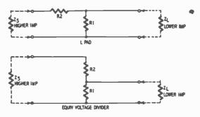
Fig. 604. The L-pad is a voltage divider.
