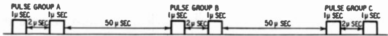
Fig. 528. A transmitted command consisting of a series of paired pulses is used with a delay line.
