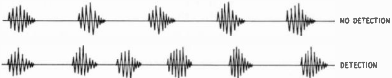
Fig. 402. Output of the superregenerative detector with and without signal. The spacing of the bursts depends upon the signal strength.
