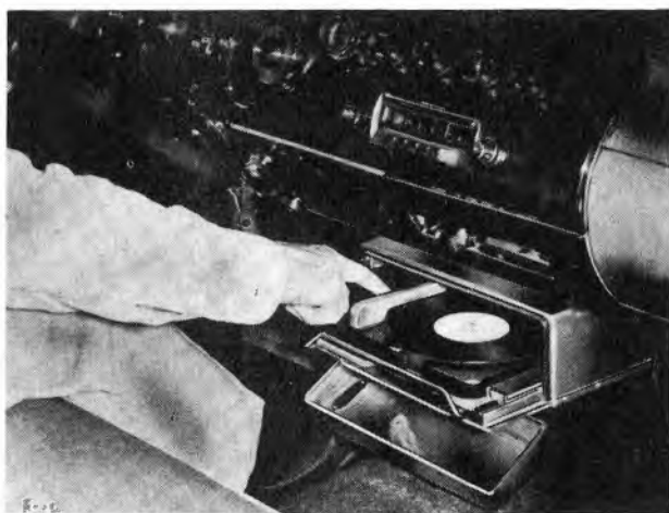
Fig. 908. Phonograph designed for use in an auto (CBS Labs).
