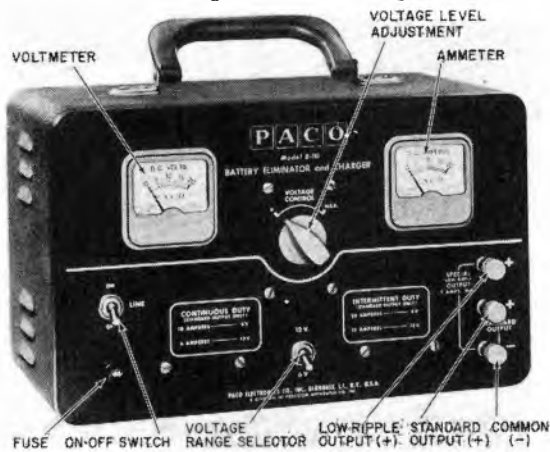
Fig. 210. Low-ripple battery eliminator. (Precision Apparatus Co.)
