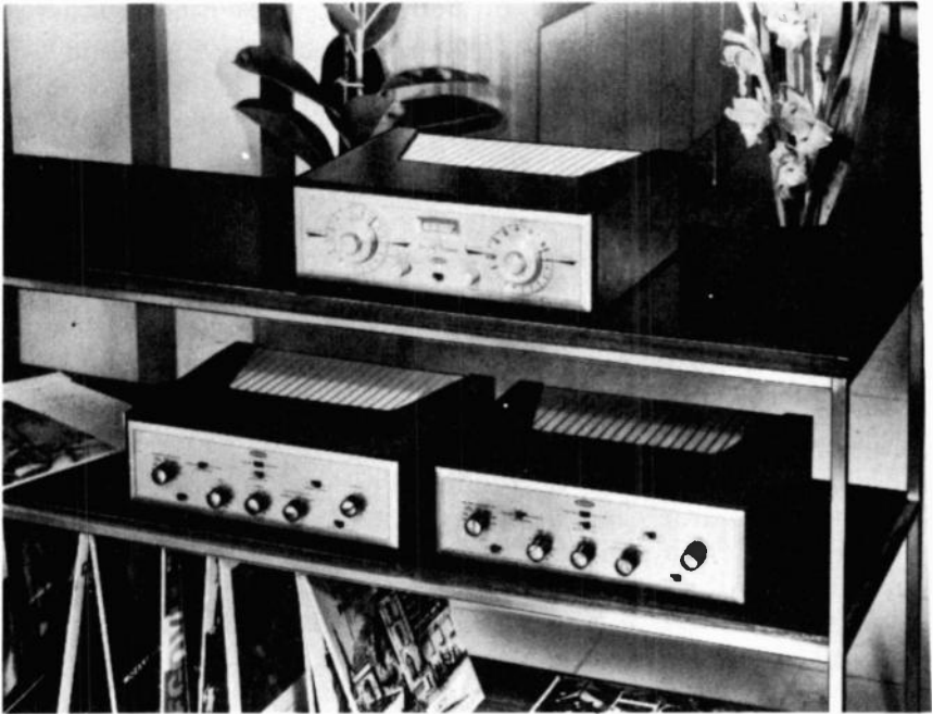
Fig. 604. The simplest and most effective way to provide adequate ventilation is by placing components on open shelves. Be careful not to obstruct vents and louvers in component cabinets. (H. H. Scott, Inc.)
