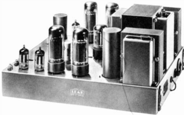
Fig. 412. The power amplifier is your hi-fi system's workhorse: (a) a typical single-channel amplifier and (b) a stereo power amplifier. Both units must be used with appropriate preamplifiers. (Upper photo: Heath Co. Lower photo: British Industries Corp.)
