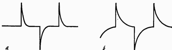
Fig. 810-a, -b. The shape of the pulse waveform can be altered by modifying the time constant of the r-c network.
