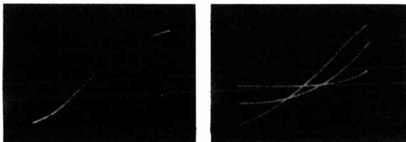
Fig. 615 (left). Photo shows the effect of running the tube into the grid current region. Fig. 616 (right). Same as Fig. 614. The use of a capacitance-coupled scope amplifier is responsible for the loss of the zero reference level.
