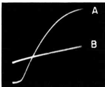
Fig. 721 (left). Effect of presence (A) and absence (B) of emitter bypass capacitor. Fig. 722 (right). Transistor amplifier circuit is stabilized when base bias voltage is obtained from a voltage divider.
