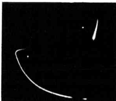
Fig. 763. P1/G1 characteristic of the multivibrator.
