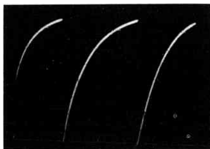
Fig. 222. Nonlinear waveform produced across C in Fig. 220.
