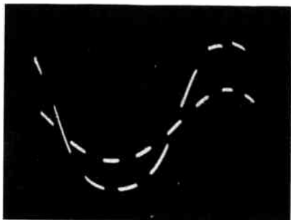
Fig. 301. By means of an electronic switch the spot successively writes two traces or parts thereof.
