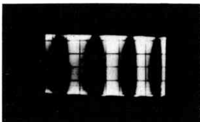
Fig. 1008 (left). 120 cps hum modulation of the CRT grid. Fig. 1009 (right). Hum modulation of the CRT grid showing display of a higher frequency.
