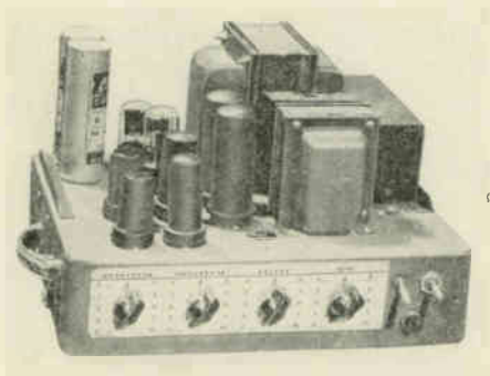
Fig. 501—The public address amplifier.
