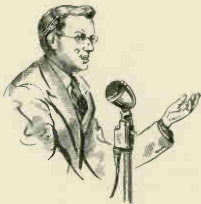
Fig. 303—Correct placement of microphone.
