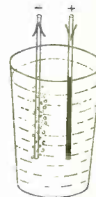
Fig. 12 - (left) Charging a 6-volt battery from a 110V. D.C. line using a variable resistance. Fig. 13 - (center) Charging a 6-volt battery using a lamp bank resistance. Fig. 14 - (right) Testing the polarity of the D.C. line with salt water.
