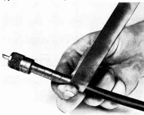
Fig. S-8. To provide extra shielding around a cable, spiral wrap with magnetic foil. (Courtesy Magnetic Shield Div., Perfection Mica Co.)
