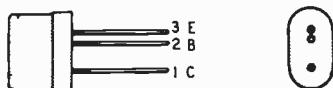
Fig. T-8. In many instances, transistor leads are not coded with color dots. If this is the case, the leads can be identified by their relative spacing.
