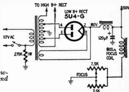
Fig. 4-P. Focus coil is part of low-voltage supply. See also Fig. 2-F and Fig. 3-F.
