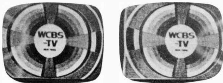
Fig. 4-F. Foldover can appear at left side of screen (pix at left) or at right side (see pix at the right).
