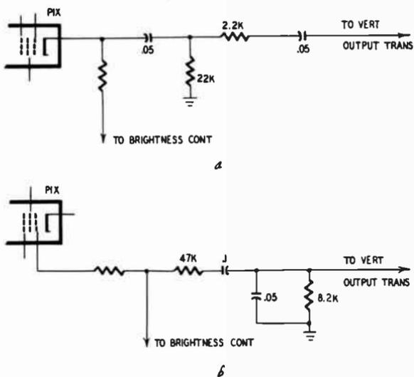
Fig. 4-R. Vertical-retrace blanking networks.
