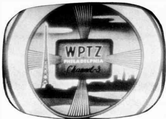
Fig. 2-B. Vertical wedges show severe bending.
