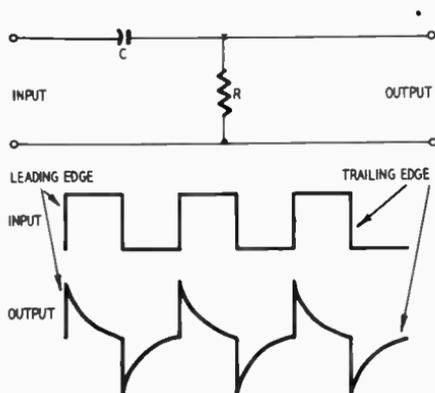
Fig. 4-D. *Effect of differentiator on horizontal-sync pulses.*
