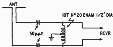
Fig. 2-1. A high-pass filter can be used to cut down interference streaks in the picture.
