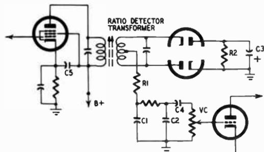
Fig. 2-R. Ratio-detector circuit. See ratio-detector check list.
