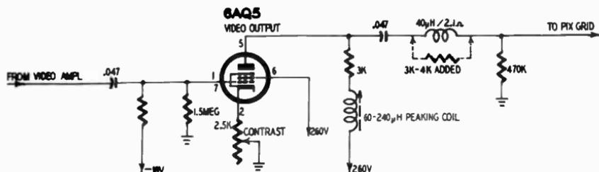
Fig. 6-R. Resistor across peaking coil helps eliminate ringing.
