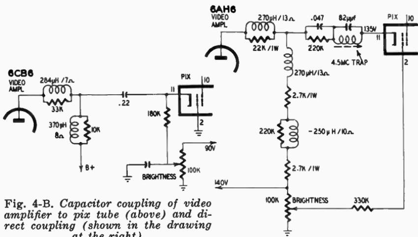
Fig. 4-B. Capacitor coupling of video amplifier to pix tube (above) and direct coupling (shown in the drawing at the right).
