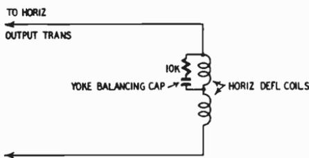
Fig. 8-R. R-C network across horizontal-deflection coil reduces ringing.
