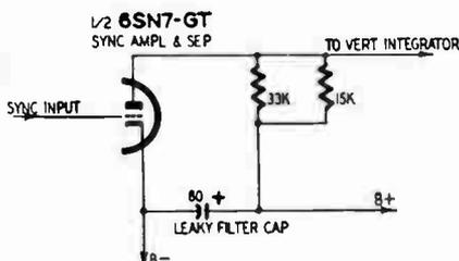
Fig. 2-V. Leaky filter capacitor can produce vertical jitter.
