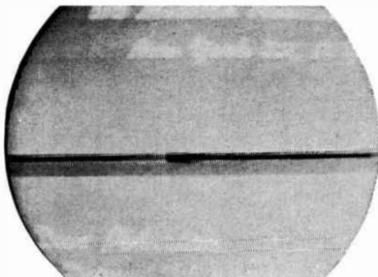
Fig. 5-S. *Blanking bar showing sync pulse.*
