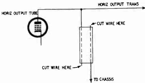
*Fig. 3-V. Capacitor made from a small piece of transmission line. Use the minimum amount of transmission line needed to increase pix width. One side of the line can connect directly to the plate cap of the horizontal-output tube. Fasten the other side of the line to the chassis.*
