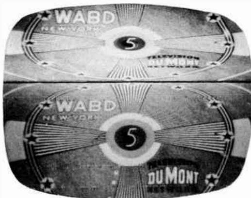
*Fig. 7-D. Double pix caused by vertical oscillator working at 30 cps.*
