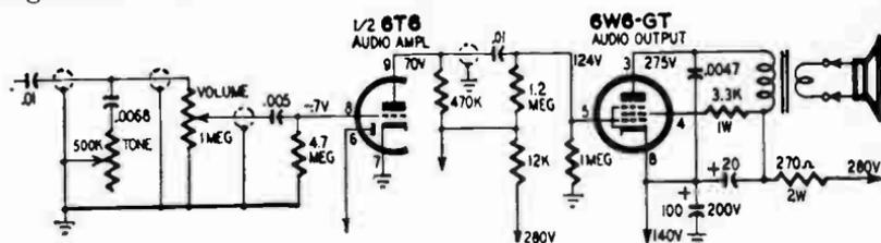
Fig. 3-N. Typical audio amplifier and output circuits.
