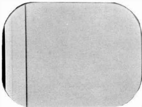
Fig. 1-B. *Appearance of Barkhausen oscillation on screen.*
