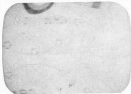
Fig. 3-K. Very poor contrast resulting from defective agc.
