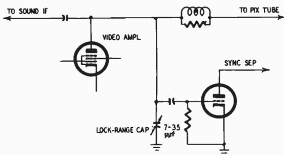
Fig. 7-P. Lock-range capacitor in sync separator circuit.
