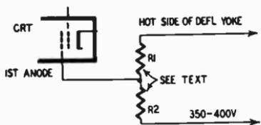
Fig. 5-F. This circuit can be added to the receiver to eliminate foldover effect.
