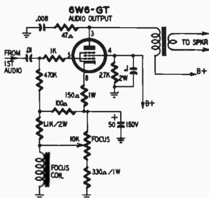
Fig. 2-F. Focus coil in audio-output circuit.
