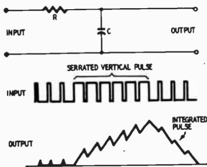
Fig. 5-I. Integrator circuit showing input and output waveforms.
