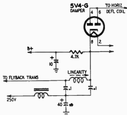
Fig. 2-N. *Damper tube and horizontal-linearity circuit.*
