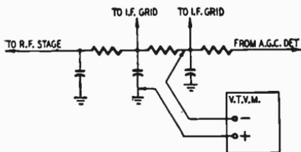
Fig. 2-A. *Measuring the agc voltage.*
