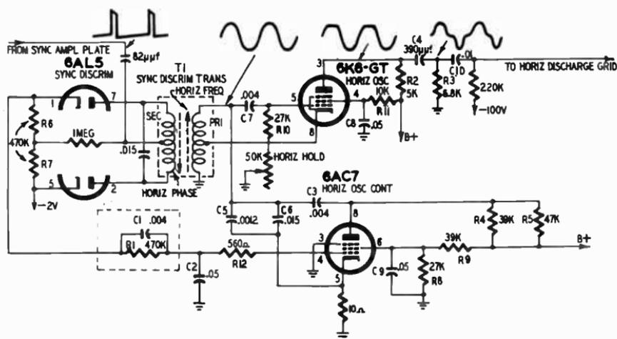
Fig. 4-H. Synchrolock horizontal-oscillator afc circuit.
