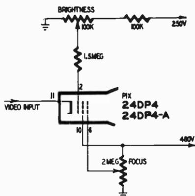
Fig. 3-F. This circuit uses electrostatic focusing.
