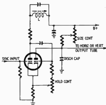
Fig. 7-R. Horizontal multivibrator may have ringing coil, L.
