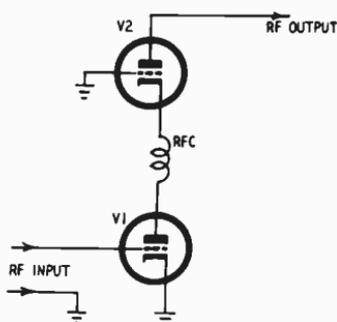
*Fig. 1-C. Simplified circuit of the cascode tuner. The two tubes are connected in series across the B+ line. Because the cathode of V2 is about 125 volts above ground, there can be a breakdown between the filament and cathode.*
