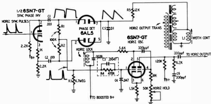
Fig. 6-H. Horizontal phase detector and multivibrator.
