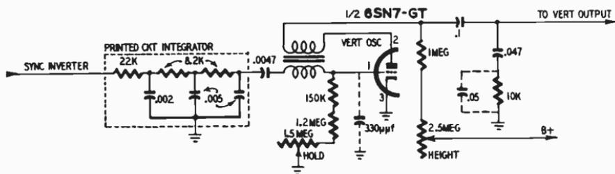
Fig. 1-1. Three-section sync integrator and its location with reference to the vertical oscillator.
