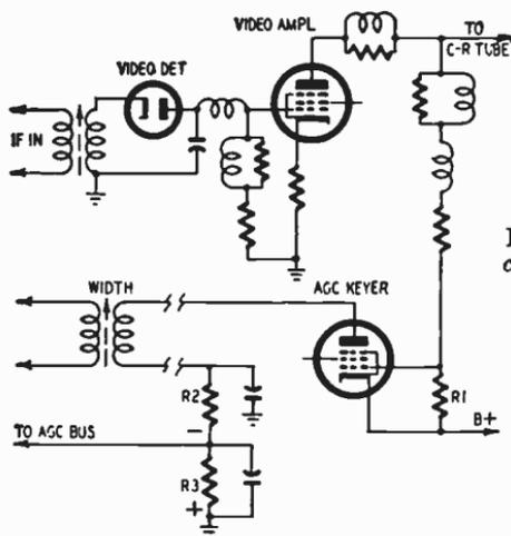
Fig. 1-K. Agc keyer circuit. Width coil is part of horizontal-output transformer.
