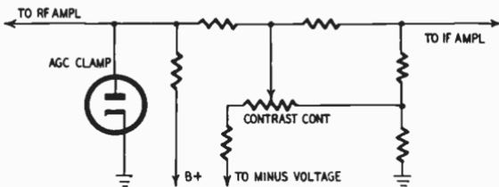
Fig. 5-A. Simple agc clamp circuit.
