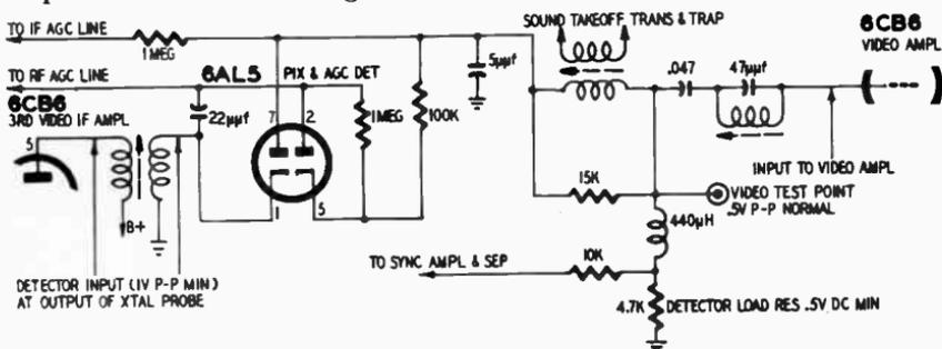
Fig. 6-C. Schematic diagram of a representative video-detector circuit.
