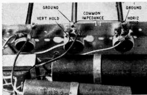
Fig. 6-D. Photo shows close positioning of vertical- and horizontal-hold controls.
