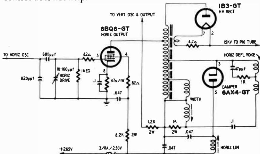
Fig. 3-H. Typical horizontal output and high-voltage circuit.
