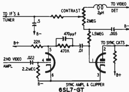
Fig. 5-C. Contrast-control circuit.
