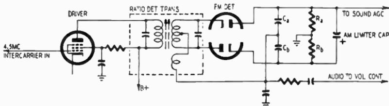
Fig. 5-B. *Typical ratio-detector circuit.*
