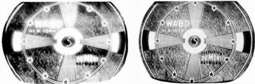
*Fig. 9-C. A photo of the face of the picture tube (before cleaning) is shown at the left. The photo at the right shows the same test pattern after the screen and the mask were cleaned. The high voltage of the picture tube seems to attract dust and will deposit a uniform layer of it over the screen.*
