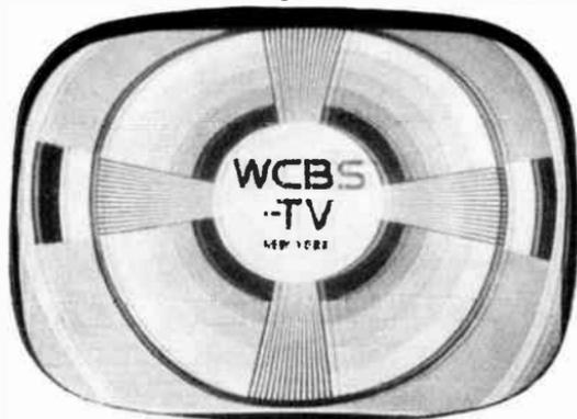
Fig. 5-R. *Pix of test pattern shows echo.*
