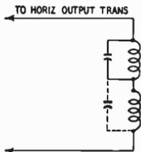
Fig. 4-V. The capacitor across one of the horizontal windings in the yoke may be misplaced, as shown by dashed lines in the drawing.
