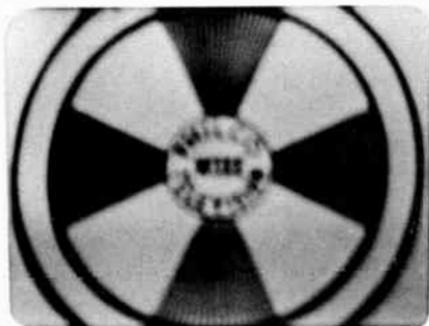
Fig 1-F. *Blurred pix due to poor focus.*
