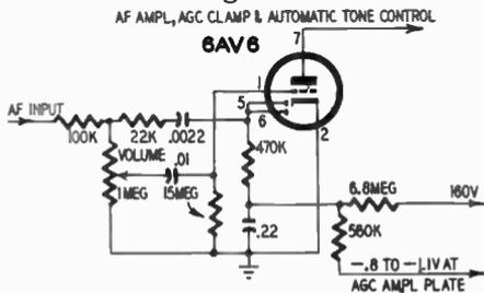
Fig. 1-A. The audio amplifier serves a number of different circuits.
