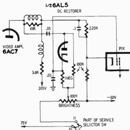
Fig. 2-D. The dc restorer acts as an automatic brightness control.
