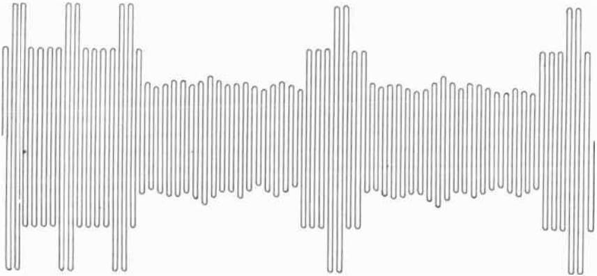
Fig. 105. The rf video carrier signal is amplitude-modulated and also carries the blanking and sync pulses.
