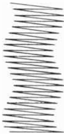
Fig. 915. Effects of hum in the horizontal oscillator and output stages. Both the raster and picture are affected.
