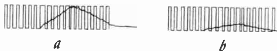
Fig. 809. Correct vertical integration (a). Poor vertical integration will produce a weak vertical sync pulse (b).
