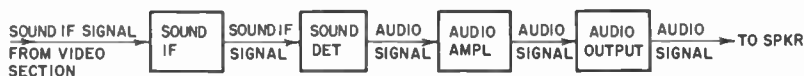
Fig 118. Block diagram of an audio section. In some sets, more than one sound if stage may be used.
