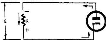
Fig. 211. Contact potential, produced by a minute current flowing through R , is serious when measuring small voltages.
