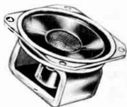
*Fig. 615. PM speakers have magnets of many shapes. Many styles are quite shallow. (Argonne Electronic Mfg. Corp.)*
