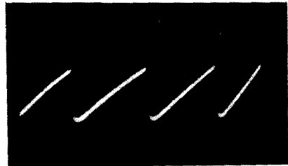
Fig. 228. With reduced amplitude, the sawtooth is almost linear.
