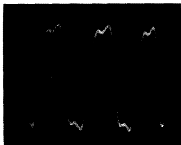
Fig. 510. 20% third harmonic. Due to different phasing, the distortion seems more severe. Note the definite symmetry of the flattened tops.
