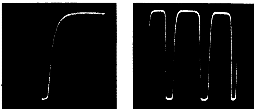
Fig. 719 (left). Overloaded transistor amplifier characteristics. Fig. 720 (right). Squared sine wave produced by an overloaded transistor amplifier.
