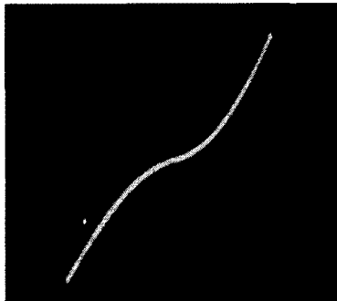
Fig. 642. Characteristic of a non-linear thyrite resistor (varistor).
