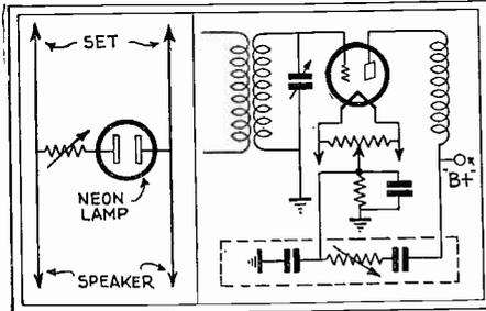
Fig. 21, left. Circuit of the static reducer.
