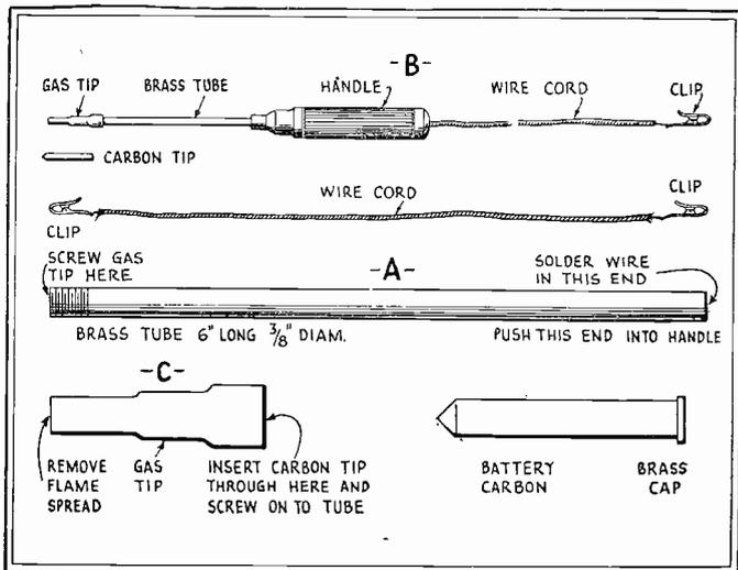
bon rod into the gas tip through the large end of the tip and screw on to brass tube.
