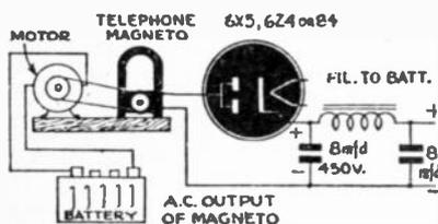
Rectifier and filter for magneto power supply.
