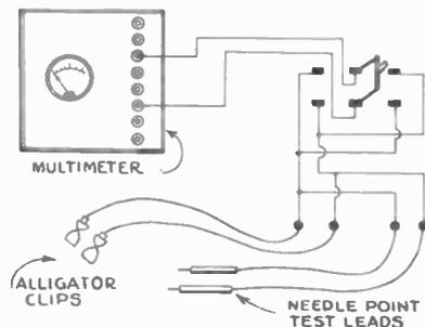
Quick reverser-switch for condenser tests.
