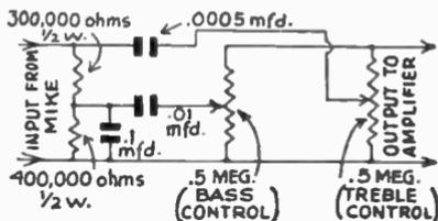
Tone control for use in pre-amplifier grid circuit.
