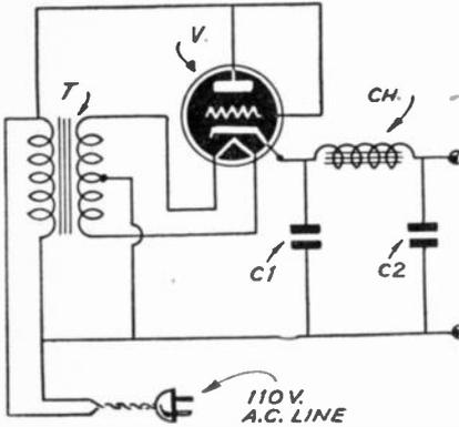
Simple power supply for test bench.
