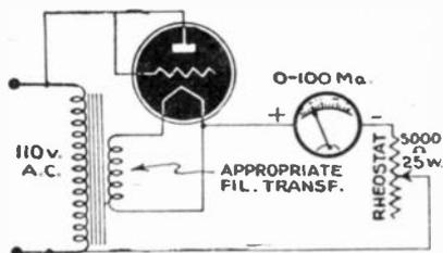
Filament emission tester of simple design.
