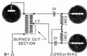
Transformer burn-out bridged by shifting connections.
