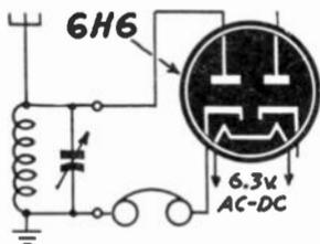
Diode detector useful in comparing crystals.
