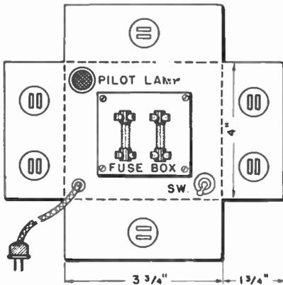
Pilot lamp and fuse for "test" outlets.
