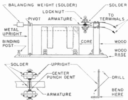
Audio transformer converted into sensitive relay.
