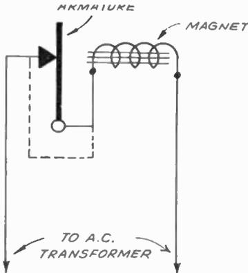
Doorbell noise eliminated by converting to a.c.
