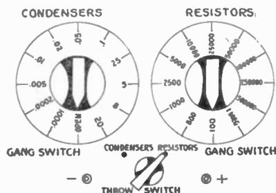
Capacity-resistor substitution box.
