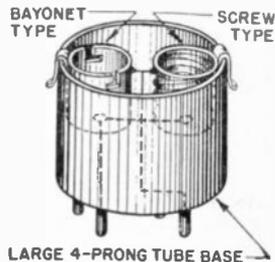
Pilot lamp tester from 4-prong tube base.
