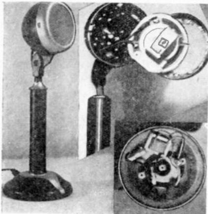
Microphone constructed from PM speaker, bicycle lamp and old telephone stand.
