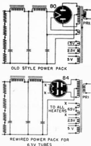
Rewiring power supply for 6.3 v tubes.
