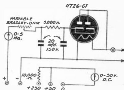
Volt-ohmmeter power supply, using 117Z6-GT tube.
