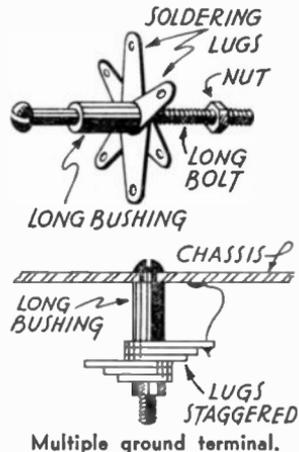
is made by using a common post consisting of soldering lugs mounted in staggered positions on a screw grounded to the chassis.—N. Z. Radiogram.
