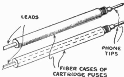
Test prods made from cartridge fuses.
