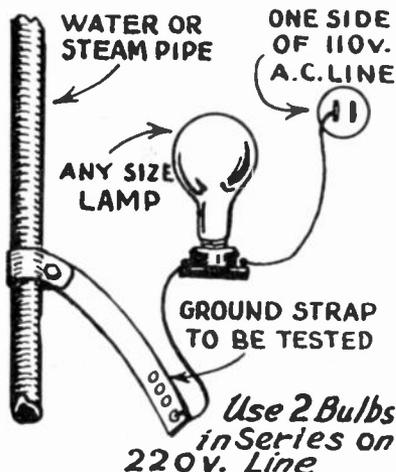
Simple ground test, using light bulb.
