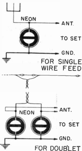
Neon lamps connected as lightning arrestors.
