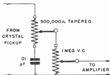
Tone and volume control for insertion between crystal pick-up and first amplifier.
