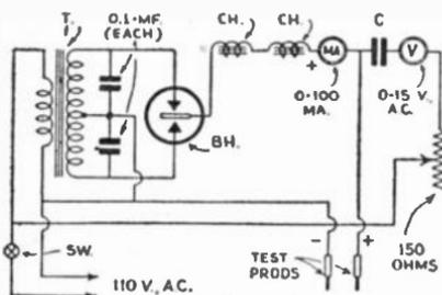
Capacity and leakage tester for condenser.
