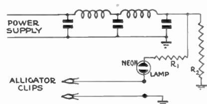
Condenser and continuity tester of simple construction, using neon lamp and resistor.
