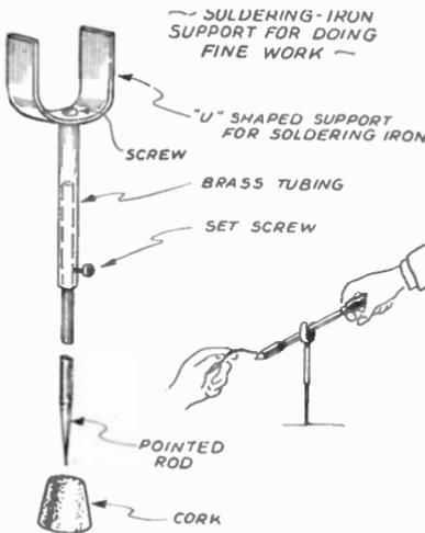
Soldering iron support for fine work.
