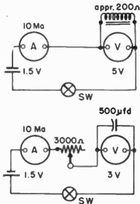
"Lag" and "lead" of current are demonstrable with these simple circuits.
