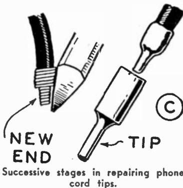
Take the wires, cut them off neatly, i.e., the insulation and the braid. Then with a sharp razor cut off the insulation so that one-quarter of an inch of the braid shows.
