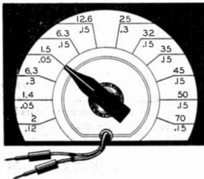
Resistance substitution box locates open filaments.
