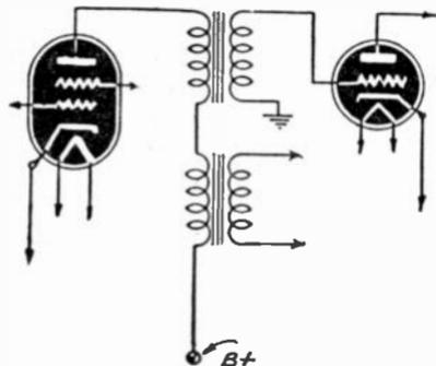
Primary of one audio transformer and secondary of another, series connected, match high plate resistance.
