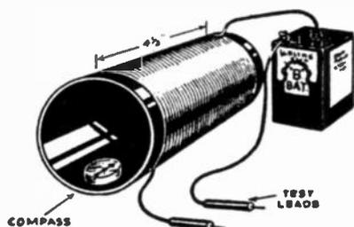
Circuit tester from coil and magnetic compass.
