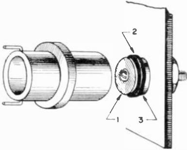
Rubber washer holds coil on chassis.
