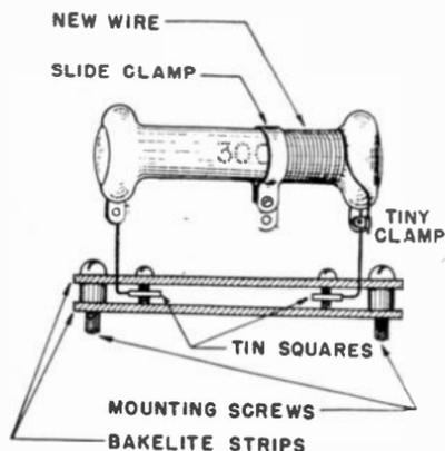
Odd-sized resistors from old insulated units.
