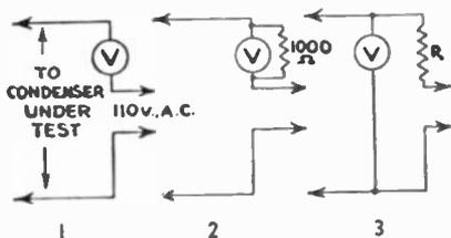
Determining condenser capacity with a.c. voltmeter.
