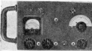
Dial at right made from protractor.
