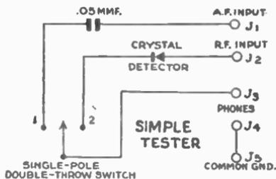
Flexible set tester for use with voltmeter.
