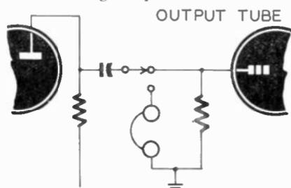
Phones connected to amplifier input circuit. connect the phones and cut out following stages, silencing the speaker. — PETER BEDROSIAN.
