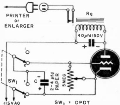
Adjustable time-interval circuit controller.
