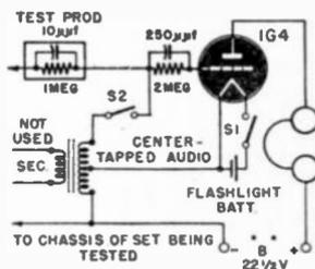
Signal tracer made from odd parts.
