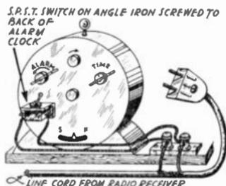
Radio cut-off switch made from alarm clock.
