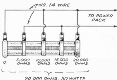
Increasing wattage capacity of resistor.
