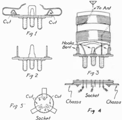
Plug-in coil from battery plug and socket.
