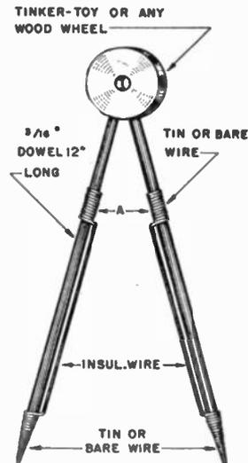
Device for shunting condensers across units under test.
