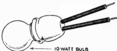
Lamp substituted for tube locates "opens".
