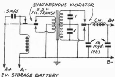
Power pack from vibrator and filament transformer.
