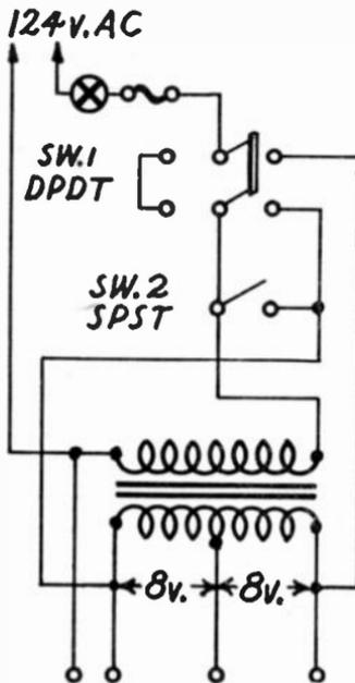
Auto-transformer hook-up to control line voltage.
