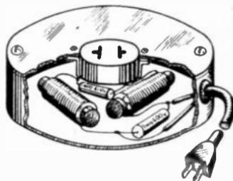
Noise filter built into outlet box.
