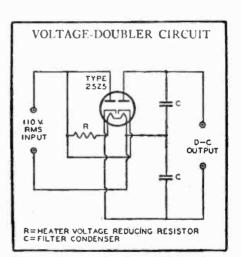
The 25Z5 may be used as a half-wave rectifier, a full-wave rectifier, or to double the output voltage when a.c. is employed.
