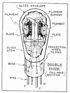
The double diode consists simply of two sets of diode elements. The 280 is the most familiar tube of this type. Similar tubes are used for detection in some special super-heterodynes.
