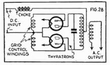
This odd circuit shows how thyratron tubes are used to convert direct current into alternating current.
