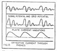
These three curves illustrate the detecting action of a three-element tube operated in the manner shown in Fig. 12, The little bumps below the time axis are practically eliminated.
