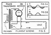
Illustrating the circuit and action of a half-wave rectifier of alternating current. Note from Fig. 5B that the output current is not continuous, but has gaps in it.
