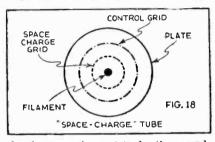
In the space-charge tetrode, the second grid is located between the filament and the regular control grid.
