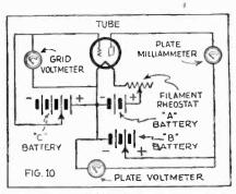
The curves of Fig. 9 may be obtained quite easily with this circuit. Only three small meters are required, in addition to the usual tilament, grid and plate batteries.
