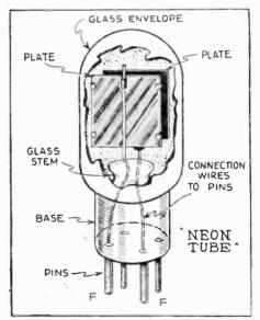
The neon tube used for television reception has two identical plates mounted parallel to each other and separated about 1/16 inch. The tube is filled with neon gas.
