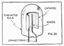
The photo-electric cell is a very simple device, consisting merely of a cathode coated with a light-sensitive material, and an abode to attract the liberated electrons. In some types, the cathode is a metallic deposit on the inside of the glass bulb.
