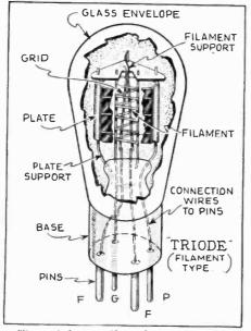
The triode or three-element tube is radio's "jack of all trades"; amplifier, detector and oscillator. In this class are the 112A, 120, 171A, 201A, 226, 230, 245, etc.
