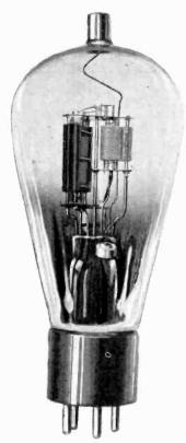
The Triple-Twin tube resembles an overgrown '45-type. Notice how the two sections are mounted on a common stem.
