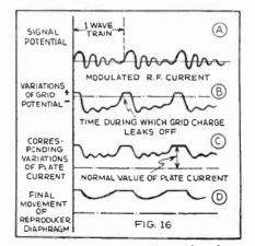
These curves show how the grid-condenser derector changes modulated radiofrequency signals into audio currents that are capable of operating earphones or other reproducers. will not leak back quickly enough, and the aforementioned blocking action occurs.
