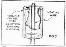
This exaggerated view shows the construction of the heated cathode used in the majority of present-day A.C. tubes. The filament in this case is merely a heater.
