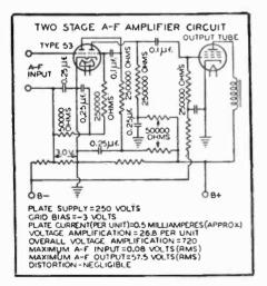
Application of the 53 tube as a class A driver. It may be also employed as a class B power stage. See chart for specifications.
