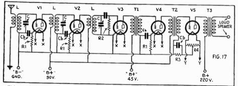
This typical tuned radio-frequency receiver shows the uses of three-element tubes as radio-frequency amplifiers. detector, and audio frequency amplifiers. The various "B" posts are intended for connection to a "B" power pack. Fila-
