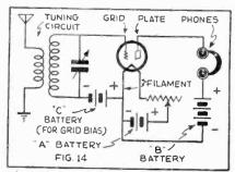
A typical grid-bias or power detection circuit. In slightly modified form, this is used in the majority of modern broadcast receivers. In A.C, sets the "C" battery is usually replaced by a biasing resistor connected in the plate return lead.
