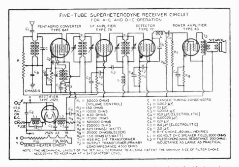
Illustrating the application of the 6.3-volt type tubes, in a typical midget receiver of the a.c.-d.c. variety. The 43 and 25Z5 are 25-volt tubes whose filament consumption is the same as that of the 6.3 volt types.
