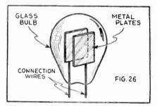
The neon tube used for television reception consists imerely of two flat metal plates, separated a short distance in a bub filled with neon gas.
