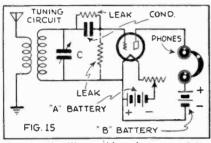
In the familiar grid-condenser system of detection, a small fixed condenser is connected in the grid lead of the tube, with a resistance of high value added in either of the two positions shown.
