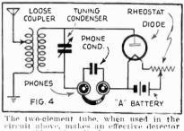
circuit above, makes an effective detector or rectifier of radio-frequency currents. This elementary circuit was used at one time for the reception of "spark" signals from old-fashioned transmitters.
