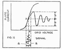
If a three-element tube is operated ou the straight section of its characteristic curve, it will faithfully reproduce any alternating current impressed on its grid. The amplitude of the plate current variations represents amplification of the signal.
