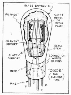
The commonest form of the diode or two-element tube is the 281 half-wave rectifier. Other diodes, built on a smaller scale, are used for detecting purposes.
