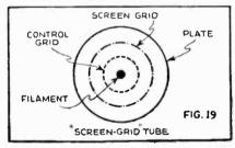
In the screen-grid tetrode, the second grid is situated between the control grid and the plate.
