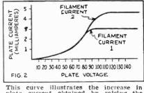
This curve illustrates the increase in plate current obtained by raising the temperature of the filament. Saturation is reached at the point where the curve flattens out at the top. The values indicated are purely relative and do not apply to any particular tube.
