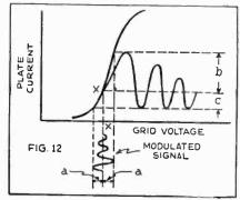
If a three-element tube is operated on the bend or "knee" of its curve, it will tend to amplify one half of the signal wave more than the other. Notice the difference in height between "b" and "c."
