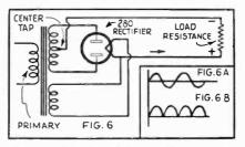
In the full-wave rectifier, both halves of the alternating current wave are used, and the output current, as shown graphically in Fig. GB, is much smoother, than the output of a half-wave rectifier.
