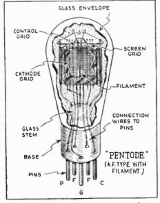
The peniodc or five-element tube has three grids. The cathode or suppressor grid, located between the screen grid and the plate, is connected internally to the center of the filament.
