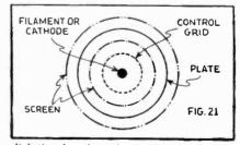
Relative location of the elements in an actual commercial screen-grid tube. The screen element completely surrounds the plate, thus shielding it thoroughly from the control grid.
