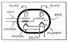
In the Triple-Twin tube, the cathode of the first section is connected internally to the grid of the second section.
