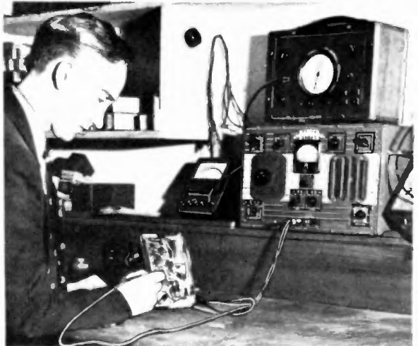
The use of the Dynalyzer (this is the instrument in the photo to which the test cord is connected).
