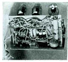
Under chassis view, showing resistor bank.
