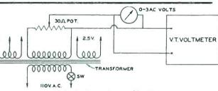
Test circuit used for calibration.
