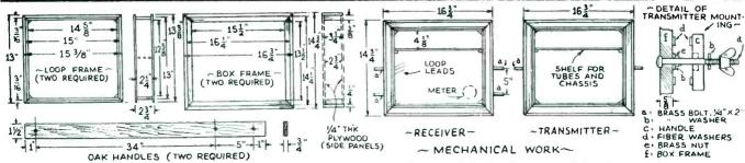
Constructional details for the loop frames, transmitter and receiver boxes, and the handles for the Fisher Treasure-Hunter.
