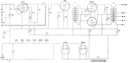
The circuit diagram of the A.C.-D.C. 4-watt Audio Amplifier.
