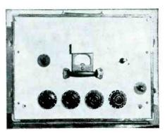
Front panel controls enable easy operation. overall gain including mixers and output pad is about 105 DB. The hum level is down 50 DB at zero level, loaded. The filament drain is .9 amps and the B battery drain is 25 mils.
