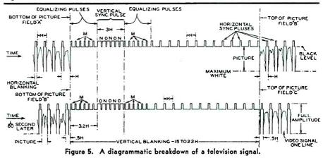
That is only 5/1000th of 1/13230th of a second, but these slopes are necessary that a wave of the proper form be supplied to the deflecting circuits of the receiver's Kinescope.
