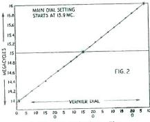
A receiver calibration. The vernier dial setting graphed.
