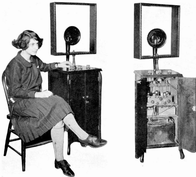
The author's "Radiotrola." This machine was built late in 1921, and is the first radio machine of its class to take on the appearance of a piece of furniture. The Radiotrola, now used in the author's home employs neither antenna nor ground, the reception being made by the loop shown in the engraving. The music, as well as entertainment, from WJZ, Newark, N. J., although twelve miles distant, comes in so loud that the sounds can be heard all over the apartment.
