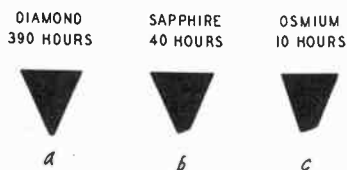
Fig. 1005-a, -b, -c. The diamond stylus has a much longer playing life than other types of needles. Although more expensive, it should be used to protect record grooves against damage by easily worn styli.
