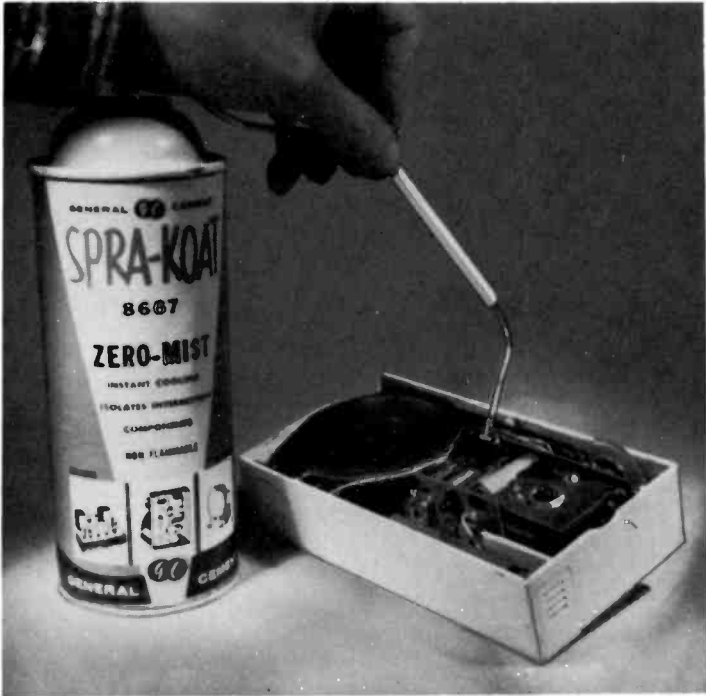
Fig. 716. Freon aerosol dispenser helps pinpoint temperature-sensitive components.
