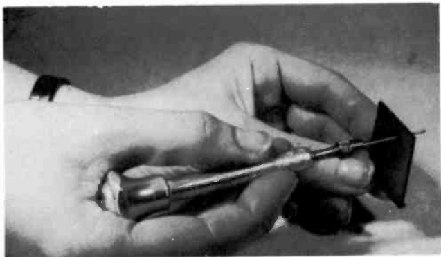
Fig. 719. The collet chuck type grip of a pin vise makes it easy to hold the smaller sizes. If the exposed end of the twist drill bit is kept as short as possible ( \frac{1}{4} inch, or so) it is possible to make small diameter holes just by carefully rotating the pin vise.
