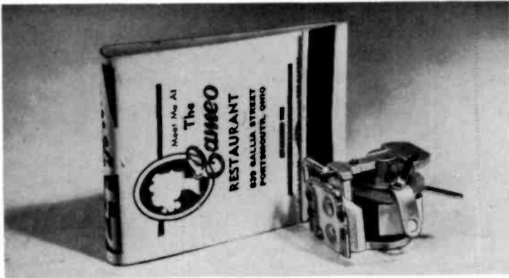
Fig. 224. The small coil of this relay draws only about one milliamperere. The wire-like contacts can handle about 200 ma.
