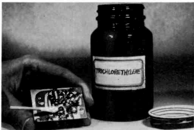
Fig. 706. Cleaning of surfaces becomes increasingly important as terminals and leads get closer together. Etching fluid residues can eat away foil conductors. Solder flux and similar substances can form leakage paths.
