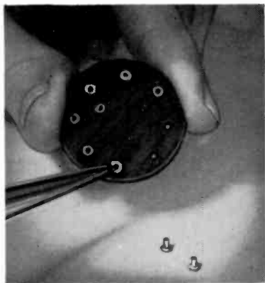
Fig. 419. Circular wafers can also be assembled into a module. Stock waste is greater than with square wafers but shape is adaptable to encapsulating in tubing.
