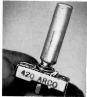
Fig. 217. Shafts can be added to many types of miniature adjustable components. Avoid heat whenever possible. Various cements can be used to do the job solder might be selected for. Use them sparingly and carefully.
