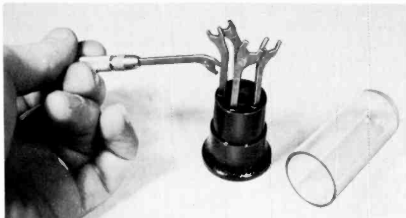
Fig. 733. Open-end wrenches can be used in places where socket wrenches can't fit.
