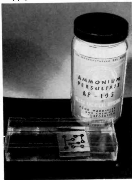
Fig. 405. Etching solution is made from powder dissolved in warm (105°F to 140°F) water. When etching, solution should be between 65°F and 70°F. Solution is good for about a week, so don't make any more than you expect to use in that time. Use non-metallic containers.
