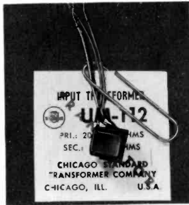
Fig. 220. Some of the smaller iron-core transformers are more like tie-tacks or shirt buttons. The smaller these transformers are made the more difficult it is to make bandpass wide. Low frequencies often suffer when size is reduced.
