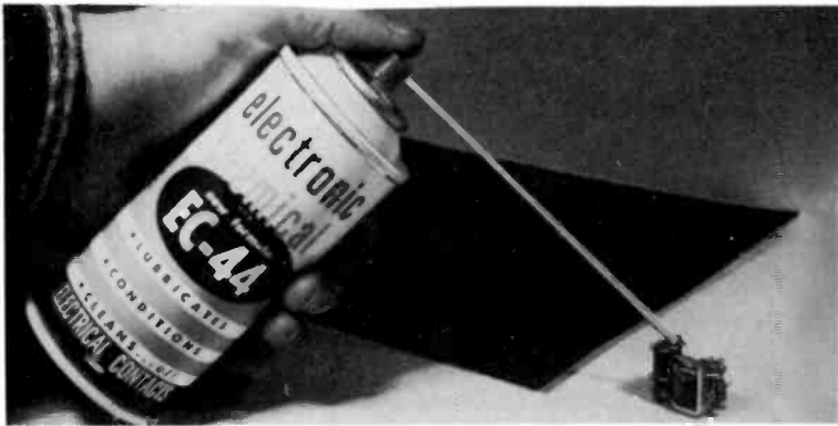
Fig. 717. Aerosol sprays are useful for cleaning all contacts and controls.
