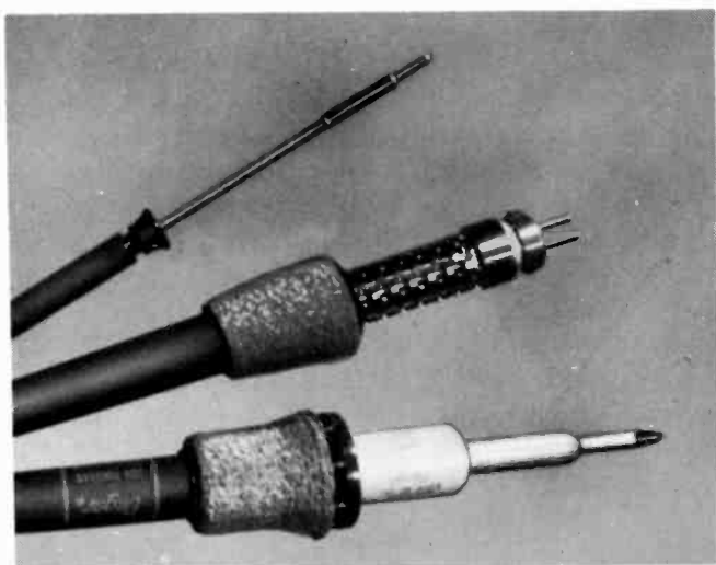
Fig. 703. Small soldering iron tips are needed to reduce the possibility of forming short-circuiting solder bridges between printed circuit conductors and contacts.
