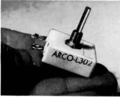
Fig. 216. Multi-turn compression-type variable capacitors may be called either trimmers or padders. Shaft can be fitted with a knob or adjusted with a screwdriver.
