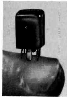
Fig. 102. The problem of miniaturizing if transformers was made easier by having only one winding tunable.
