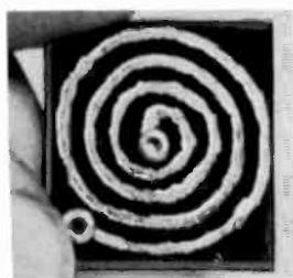
Fig. 222. Painted subminiature inductors are useful for low values of inductance.
