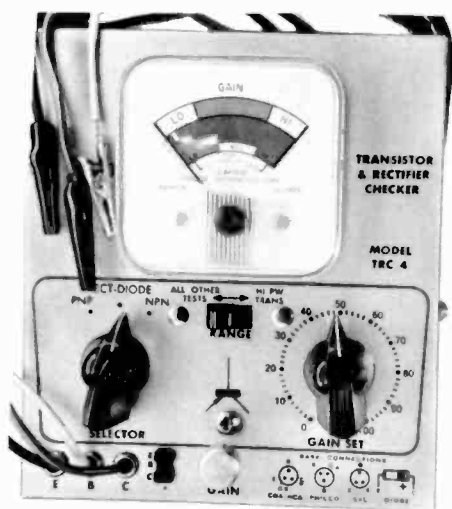
Semiconductor diode testing has been simplified by the Diode Transistor tester.
