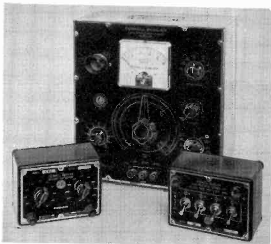
Resistor-capacitor analyzer and capacitor decade boxes are useful in finding and substituting defective filters and bypass networks.
