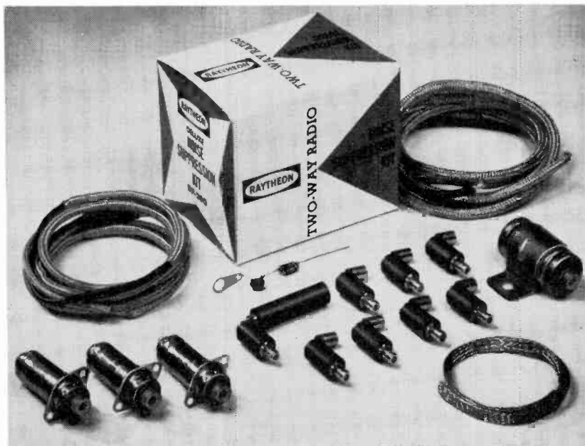
This do-it-yourself ignition noise suppression kit can be used to advantage with any internal combustion engine where it interferes with the reception on broadcast, marine or Citizens bands. It includes suppressors, capacitors, an R-C network and shielded generator wiring. (Raytheon Company)
