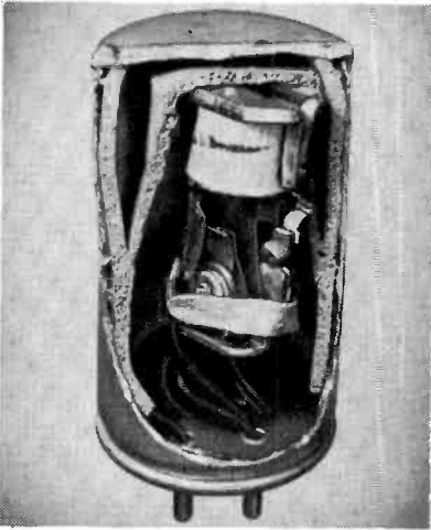
Cutaway of vibrator shows molded foam rubber used to silence vibrator. Leads are kept in place with a rubber band. (Gem Electronics)
