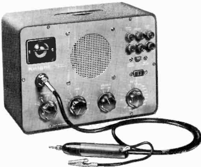
Fig. 511. Signal tracer is extremely useful in servicing receivers. (Allied Radio Corp.)
