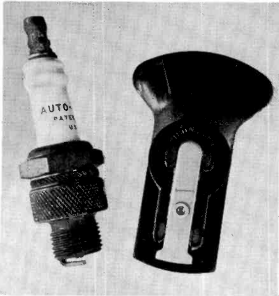
Excessive electrode gap in the spark-plug (left) or corroded top connector can help generate excessive noise just as wear and burning of the rotor tip or a dirty or poor contact will at the center contact of the rotor. These normal-wear points can create noise before hard-starting or engine performance is affected.
