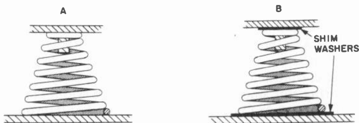
Fig. 509-a,-b. If one or more corners of the chassis are not high enough (a) shim washers can be added (b).
