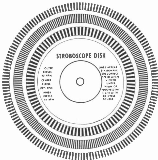
Fig. 202. Typical stroboscope disc. This is a simple and effective means for checking the speed of the motor.
