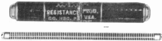
Fig. 413. Multiplier resistors used in high-voltage probes.
