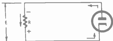
Fig. 211. Contact potential, produced by a minute current flowing through R , is serious when measuring small voltages.
