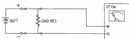
Fig. 1003. Method of testing battery voltage.
