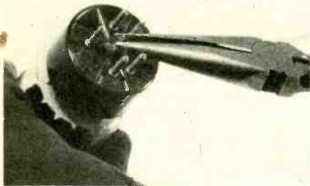
Break off the black tube-locator pin and the glass tip with some long nose pliers.
