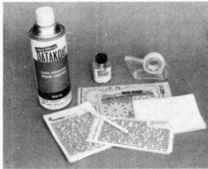
2. You will need spray and brush-on protective coating, plastic tape, various types of rub-on lettering and designs, and a burnishing tool (the white cylinder) to effect the transfer of the letters from the carrier sheet to a project's front panel.
