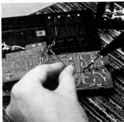
**Cracked PC Board.** You may find a cracked PC board after careless handling or after an accident. When the calculator is accidentally dropped or knocked around, check for broken wiring connections or a cracked PC board. In one particular instance, a pocket calculator was accidentally dropped upon the cement floor of a garage and the cover accidentally run over by a car. The only damage incurred was a broken corner of the cal-
