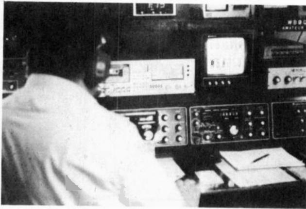
This proud exhibitor at an SSTV hamfest shows off the sophisticated gear used in the pursuit of his hobby. On the right side of the table is the transmitter, to the left an audio amplifier with a cassette deck, and above the amplifier is the monitoring CRT screen. Below is a view of a ham shack with all of the equipment fired up and an SSTV QSL broadcast on the CRT display. As equipment becomes available, Amateur SSTV will grow.
