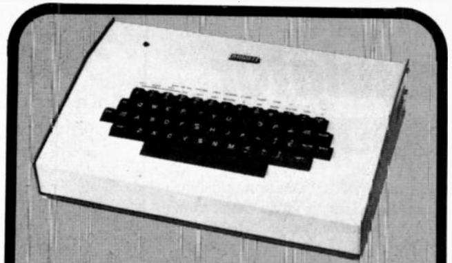
The Robot keyboard is used to enter ASCII coded characters to the SSTV transmitter for broadcast over the air. This arrangement is used instead of more expensive camera.
