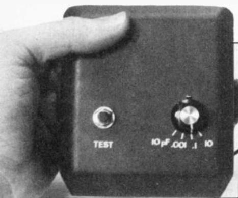
This digital capacitance meter is a cinch to use; just clip the leads to the capacitor, select the right range and push the TEST button.
