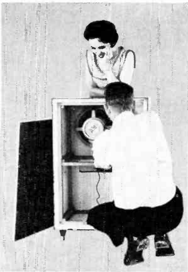
Final steps in building the Club Sandwich are mounting speaker and putting the back in place.
