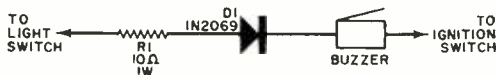
Light Minder uses three components; R1 is omitted in 6-volt cars, leads reversed for positive ground.
