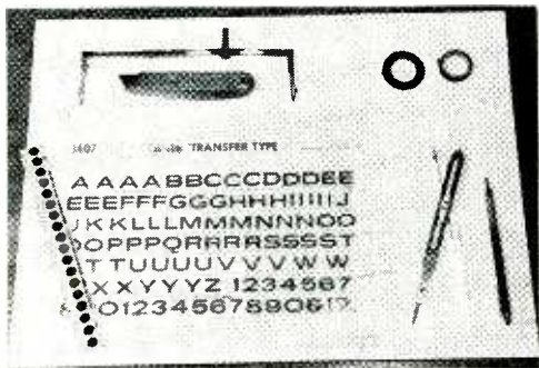
Fig 2. Materials you need for making a new face include instant transfer letters, a beam compass, \frac{3}{8} " printed circuit dots, \frac{1}{8} "- and 1/16 "-wide black printed circuit tape, and white illustration board.
