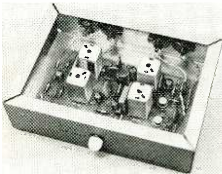
Fig. 9. A printed circuit board or any other standard wiring technique can be used. All components are mounted on one side. Keep transistors about \frac{1}{4} " above the board, or install in sockets.
