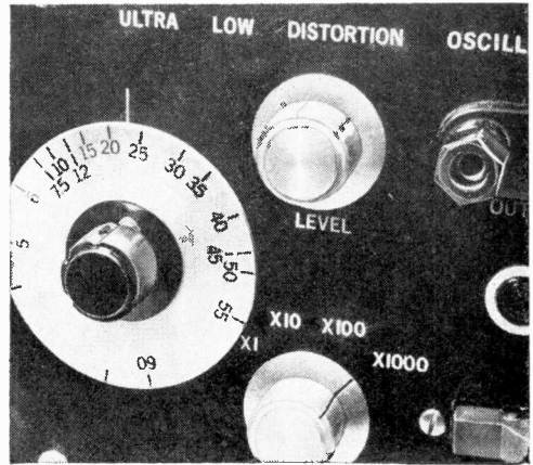
Calibration markings on sweep-frequency control dial (left in above photo) are obtained by interpreting Lissajous patterns produced by 60-Hz line and oscillator output frequencies fed into an oscilloscope.
