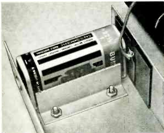
Fig. 3. For installation of 22.5-volt battery, one side of chassis box must be dimpled to accept negative contact (above). Positive pole connection consists of brass shim (left), insulated from box with fiber paper. Small L-bracket holds battery in upright position. Note the wire connected to shim.
