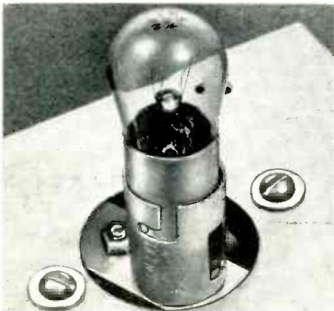
Ferrule of bayonet socket protrudes through a hole in top of box and is fastened with machine screws.
