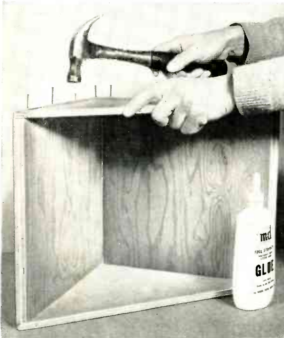
Fig. 2. Liberal bead of white glue between joined members helps to rigidize enclosure and provides air seal. Finishing nails anchor members together.
