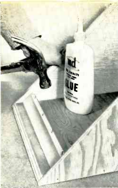
Fig. 3. Side cleats are miter cut at 45° angles; then glued and nailed to sides, 1/2" in from front.
