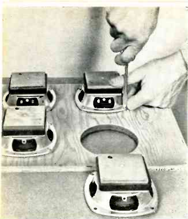
Fig. 5. Fasten loudspeakers to speaker mounting board with #8 x 1/2" pan-head sheet metal screws.
