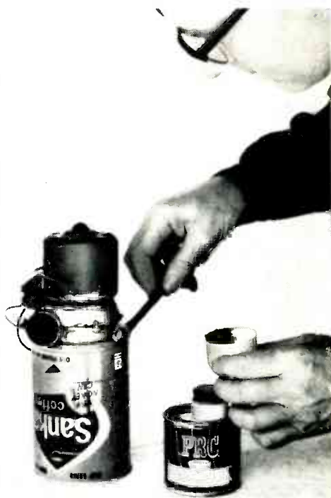
Fig. 2. The small fan is cemented to its hole in top of can. Make sure that the joint is airtight.
