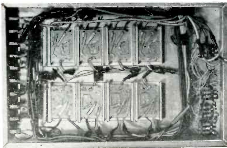
When mounting a number of dimmers in one chassis, make sure that sufficient heat sink area is provided to enable each to operate at a safe temperature.
