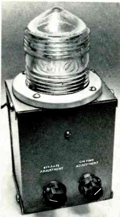
The Fresnel lens assembly bolts to the top of the chassis box with four sets of #6 machine hardware.
