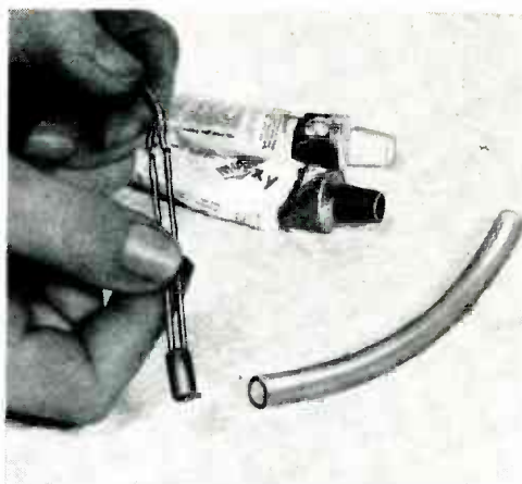
Taped-end neoprene tubing serves as the form when assembling the probe elements with hard-set epoxy.
