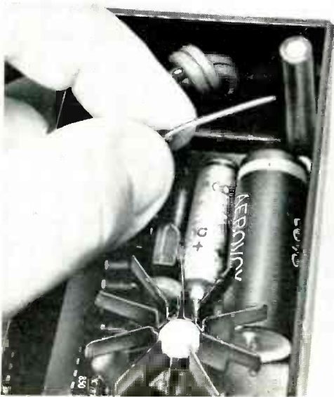
Fig. 4. Bare wire can be either wrapped around cover hold-down screw or clamped in screw receptacle.
