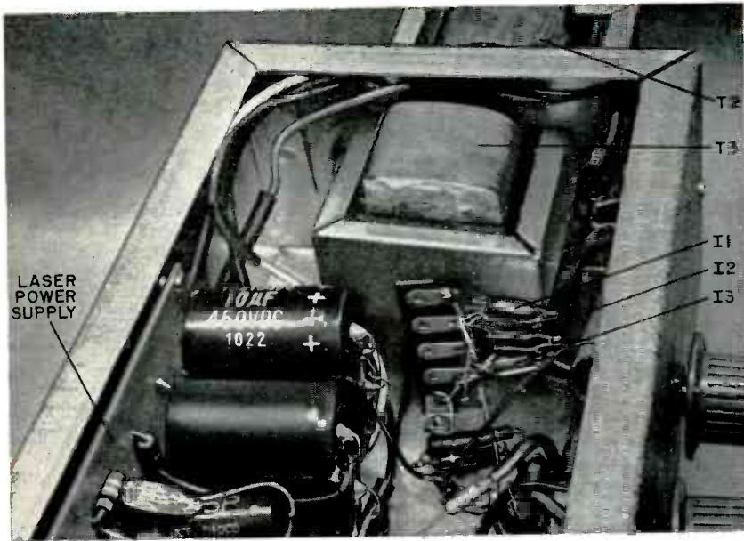
Internal layout of the prototype transceiver (above) showing the laser power supply mounted on one wall with the rest of the components occupying the remaining space. The internal arrangement of the telescope electronics (shown below) shows the modulator tube and its associated components arranged within its smaller metal enclosure.
