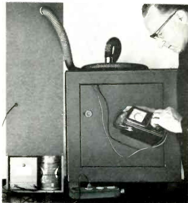
Fig. 9. The front door is open at the bottom of the cabinet to allow for air intake and observation of the indicator lamp. To prevent operation when the door is open, a TV “cheater” cord and socket are engaged when door is closed.
