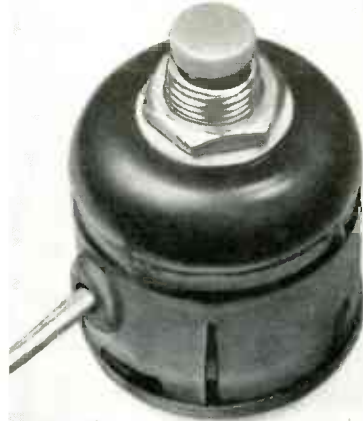
Fig. 6. Amphenol shell accommodates remote actuating switch. Cable should be routed through a grommet-lined hole.
