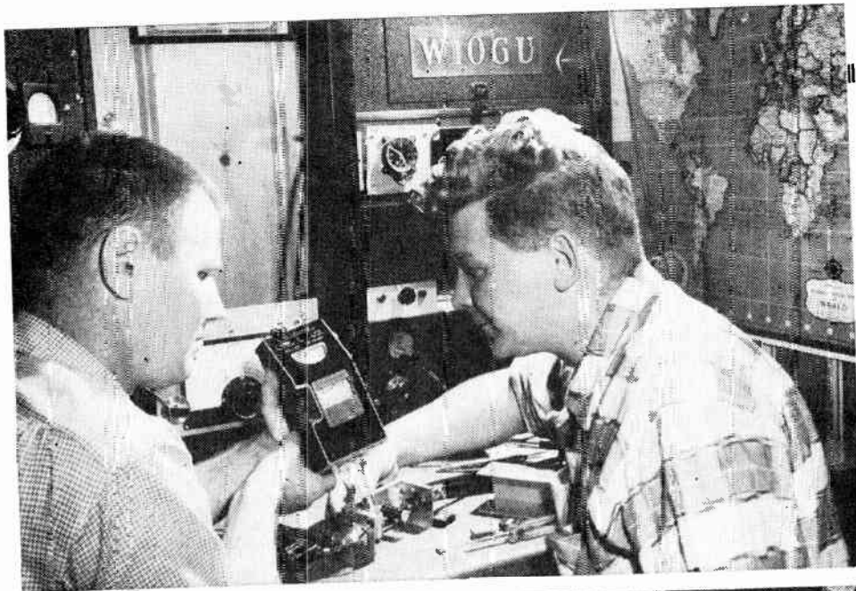
The authors tune up the tiny transistorized transmitter with grid-dip meter prior to going on air. (Right) Gus Fallgren keys the transmitter whose power source is 6 v. battery.
