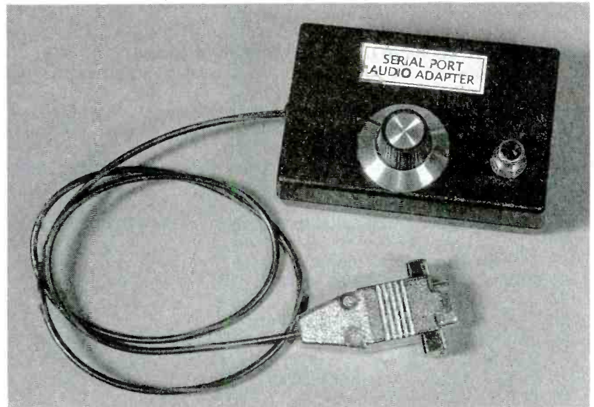
FIG. 3—THE ASSEMBLED UNIT is compact and attractive. An even smaller case than the one shown here could also be used.
