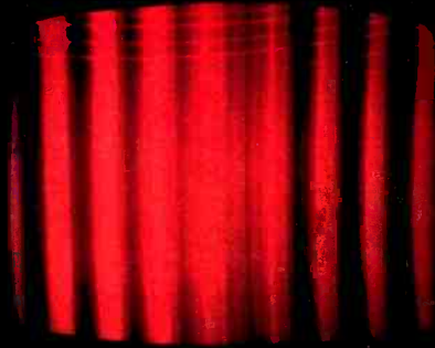
HUE CONTROL Proper setting blends sixth bar into background. Kill green and blue guns to obtain this display.
