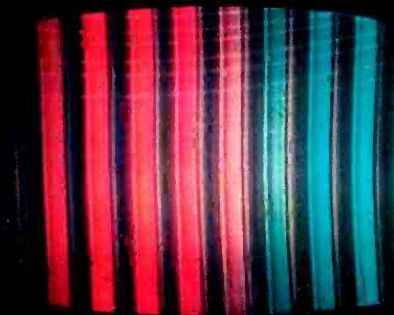
HUE CONTROL Proper setting blends sixth bar into background. Kill green and blue guns to obtain this display.
