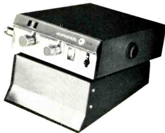
This base-station transceiver is mounted atop housing that is used for a.c. power supply and speaker.
