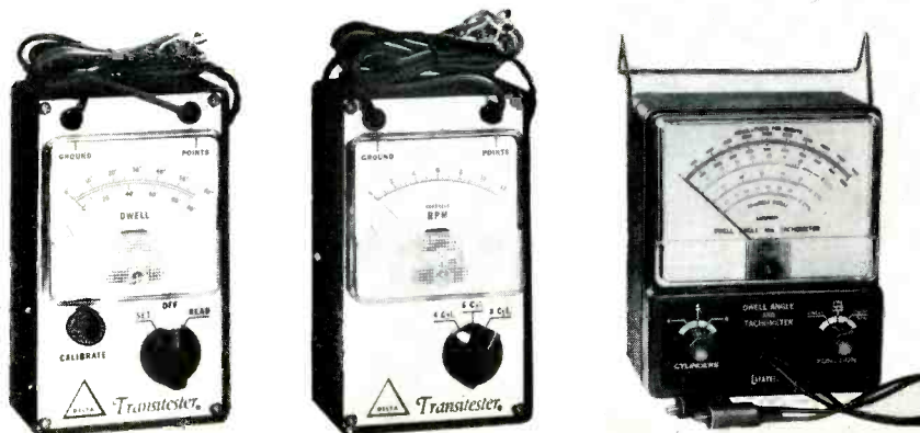
Examples of typical dwell meter (far left) and tachometer (center) are these Delta D-1000 and T-1000. Such units show how long breaker points stay closed, and speed of engine. A combination automotive dwell meter and tachometer (right) is this Lafayette No. 11-0101 unit.
