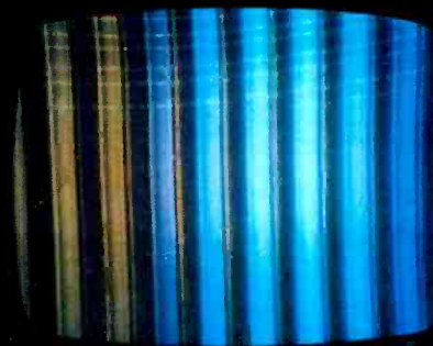
DEMODULATORS INOPERATIVE Defective Z (or B-Y) demodulator shows up mostly as loss of blues (top); predominant loss of reds (above) can be traced to troublesome X (or R-Y) demodulator. Absence of the red or blue colors also causes a loss of the green.
