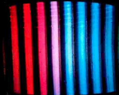
COLOR BAR PATTERN Normal display is indication of proper operation of phase, matrix, and other circuits.
