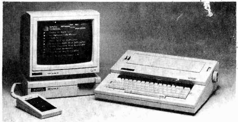
Complete SCM word processor system has four parts. They are, left, 12-inch monitor atop CPU (Central Processing Unit) right, combination typewriter/printer, and small control unit. List-price about $1000, however, can be purchased for as low as $800.
