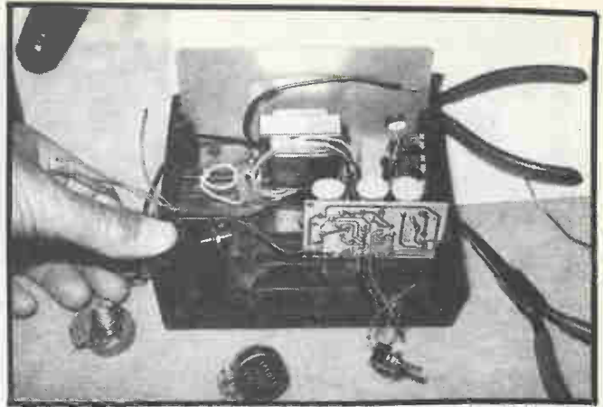
Figure 3: Select a cabinet big enough for all parts. Here parts are jammed together in a project case that is too small.
