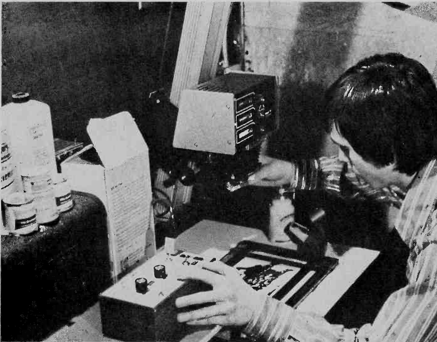
IC-design photo timer features backlighted digit-set dials, pushbutton start and stop buttons, and safelight control. Modern circuitry provides high accuracy and repeatability over the 1 to 119 second timing range. Home darkroom using our photo timer is equipped with Omega B color enlarger.
