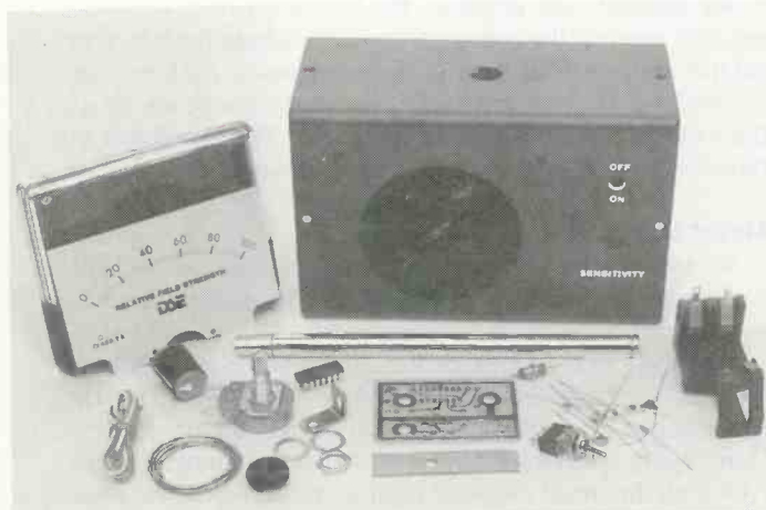
The Field-Strength Meter Kit is an old-fashioned type. Nothing is pre-assembled. Even the meter's special pre-calibrated scale must be installed by the builder.
