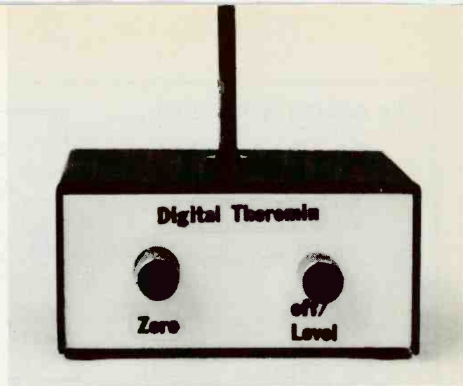
This frontal view of the Digital Theremin shows the location of the panel-mounted controls. Also notice that the antenna, beside going through a grommet on the printed-circuit board, protrudes through a second grommet mounted top-center of the enclosure, lending support to the installation.
