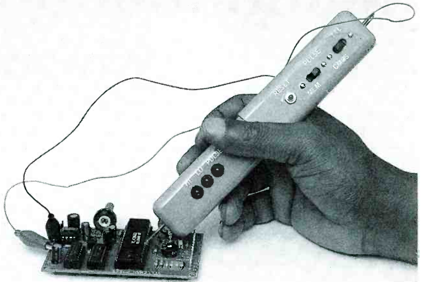
Because operational power for the Experimenter's Logic Probe is derived from the circuit-under-test, you must connect the alligator clips of its power-supply leads to the +V and ground buses of the circuit to be monitored.
