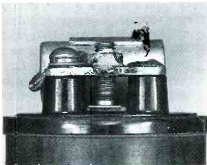
The points on the coil should be just barely touching. The capacitor (once called a condenser) is visible just behind them. To avoid damaging yourself or the coil, make no attempt to adjust the points while the coil is operating.
