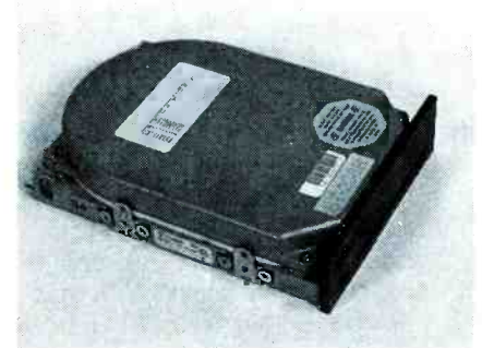
Half-height hard-disk drives designed to fit into one of the slots intended for floppy disk drives, can give you super storage in a very tiny space. Technology has really changed!
